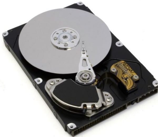
Hard Drive (cover removed)
