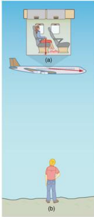
Figure 3.34: The motion of a coin dropped inside an airplane as viewed by two different observers. (a) An observer in the plane sees the coin fall straight down. (b) An observer on the ground sees the coin move almost horizontally.
