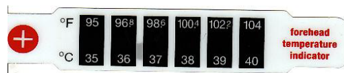
Figure 13.2: Each of the six squares on this plastic (liquid crystal) thermometer contains a film of a different heat-sensitive liquid crystal material. Below 95°F, all six squares are black. When the plastic thermometer is exposed to temperature that increases to 95°F, the first liquid crystal square changes color. When the temperature increases above 96.8°F the second liquid crystal square also changes color, and so forth. (credit: Arkrishna, Wikimedia Commons)
