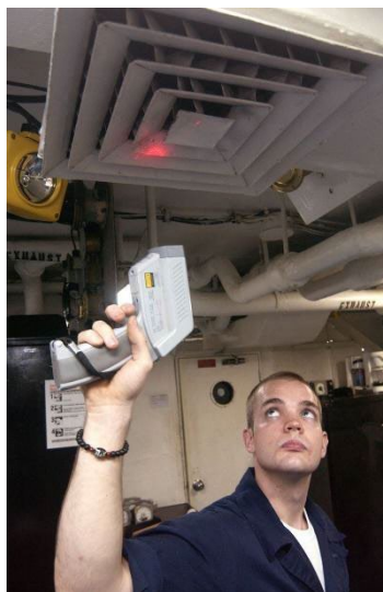
Figure 13.3: Fireman Jason Ormand uses a pyrometer to check the temperature of an aircraft carrier's ventilation system. Infrared radiation (whose emission varies with temperature) from the vent is measured and a temperature readout is quickly produced. Infrared measurements are also frequently used as a measure of body temperature. These modern thermometers, placed in
