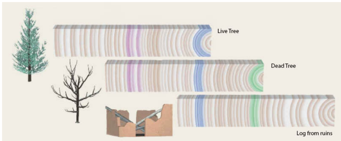
Figure 3: Long tree ring chronologies can be constructed by matching overlapping patterns of different trees.
