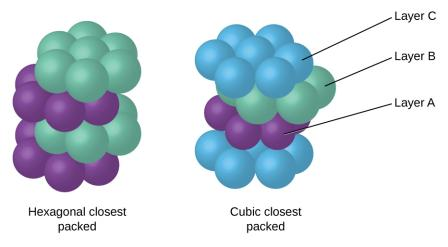
**Figure 10.54** In both types of closest packing, atoms are packed as compactly as possible. Hexagonal closest packing consists of two alternating layers (ABABAB...). Cubic closest packing consists of three alternating layers (ABCABCABC...).
