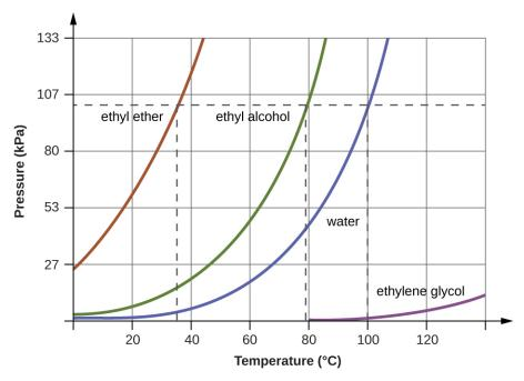
**Figure 10.24** The boiling points of liquids are the temperatures at which their equilibrium vapor pressures equal the pressure of the surrounding atmosphere. Normal boiling points are those corresponding to a pressure of 1 atm (101.3 kPa.)
