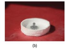
**Figure 19.11** (a) This magnetic levitation train (or maglev) uses superconductor technology to move along its tracks. (b) A magnet can be levitated using a dish like this as a superconductor. (credit a: modification of work by Alex Needham; credit b: modification of work by Kevin Jarrett)
