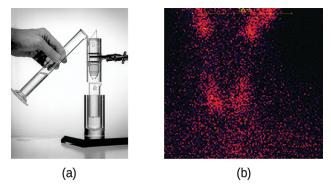
**Figure 20.25** (a) The first Tc-99m generator (circa 1958) is used to separate Tc-99 from Mo-99. The  ${\rm MoO_4}^{2-}$  is retained by the matrix in the column, whereas the  ${\rm TcO_4}^-$  passes through and is collected. (b) Tc-99 was used in this scan of the neck of a patient with Grave's disease. The scan shows the location of high concentrations of Tc-99. (credit a: modification of work by the Department of Energy; credit b: modification of work by "MBq"/Wikimedia Commons)
