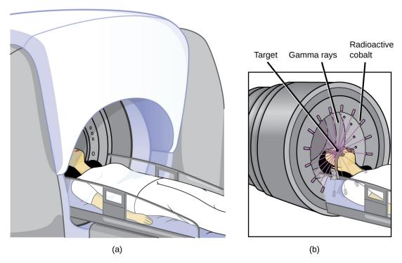
**Figure 20.26** The cartoon in (a) shows a cobalt-60 machine used in the treatment of cancer. The diagram in (b) shows how the gantry of the Co-60 machine swings through an arc, focusing radiation on the targeted region (tumor) and minimizing the amount of radiation that passes through nearby regions.
