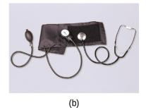
**Figure 8.6** (a) A medical technician prepares to measure a patient's blood pressure with a sphygmomanometer. (b) A typical sphygmomanometer uses a valved rubber bulb to inflate the cuff and a diaphragm gauge to measure pressure. (credit a: modification of work by Master Sqt. Jeffrey Allen)
