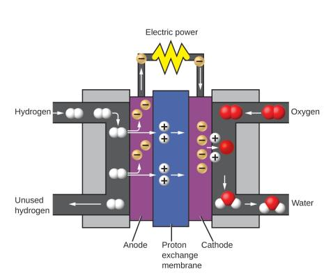
**Figure 1.16** A fuel cell generates electrical energy from hydrogen and oxygen via an electrochemical process and produces only water as the waste product.
