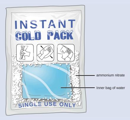
**Figure 9.16** An instant cold pack consists of a bag containing solid ammonium nitrate and a second bag of water. When the bag of water is broken, the pack becomes cold because the dissolution of ammonium nitrate is an endothermic process that removes thermal energy from the water. The cold pack then removes thermal energy from your body.
