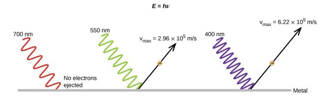
**Figure 3.11** Photons with low frequencies do not have enough energy to cause electrons to be ejected via the photoelectric effect. For any frequency of light above the threshold frequency, the kinetic energy of an ejected electron will increase linearly with the energy of the incoming photon.
