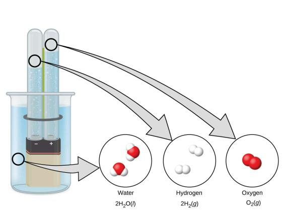
**Figure 1.15** The decomposition of water is shown at the macroscopic, microscopic, and symbolic levels. The battery provides an electric current (microscopic) that decomposes water. At the macroscopic level, the liquid separates into the gases hydrogen (on the left) and oxygen (on the right). Symbolically, this change is presented by showing how liquid  $H_2O$  separates into  $H_2$  and  $O_2$  gases.
