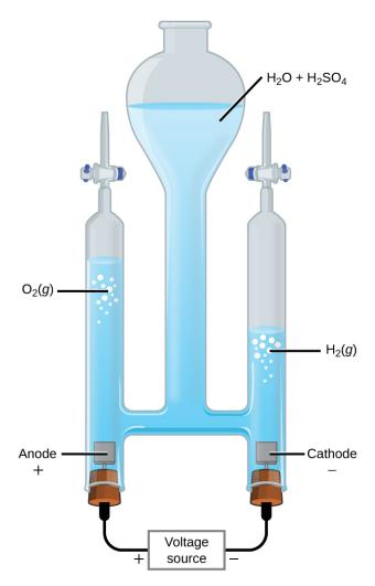
**Figure 16.19** The electrolysis of water produces stoichiometric amounts of oxygen gas at the anode and hydrogen at the anode.
