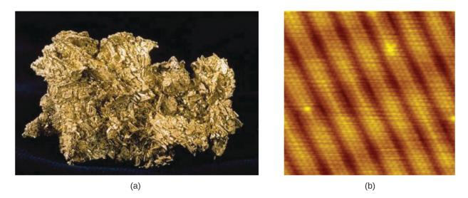
**Figure 1.12** (a) This photograph shows a gold nugget. (b) A scanning-tunneling microscope (STM) can generate views of the surfaces of solids, such as this image of a gold crystal. Each sphere represents one gold atom. (credit a: modification of work by United States Geological Survey; credit b: modification of work by "Erwinrossen"/Wikimedia Commons)
