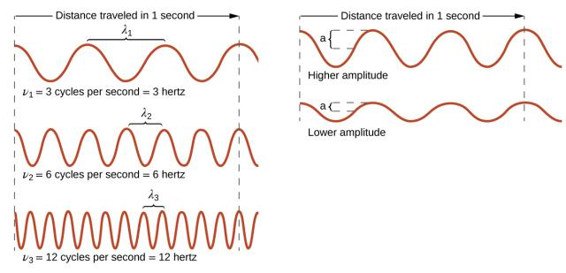
**Figure 3.2** One-dimensional sinusoidal waves show the relationship among wavelength, frequency, and speed. The wave with the shortest wavelength has the highest frequency. Amplitude is one-half the height of the wave from peak to trough.
