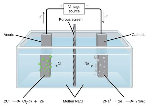
**Figure 16.18** Cells of this sort (a cell for the electrolysis of molten sodium chloride) are used in the *Downs process* for production of sodium and chlorine, and they typically use iron cathodes and carbon anodes.
