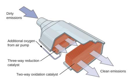
**Figure 17.26** A catalytic converter allows for the combustion of all carbon-containing compounds to carbon dioxide, while at the same time reducing the output of nitrogen oxide and other pollutants in emissions from gasoline-burning engines.
