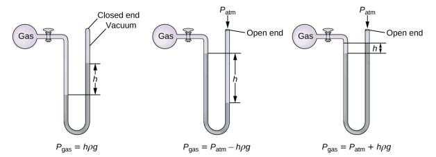
**Figure 8.5** A manometer can be used to measure the pressure of a gas. The (difference in) height between the liquid levels (*h*) is a measure of the pressure. Mercury is usually used because of its large density.
