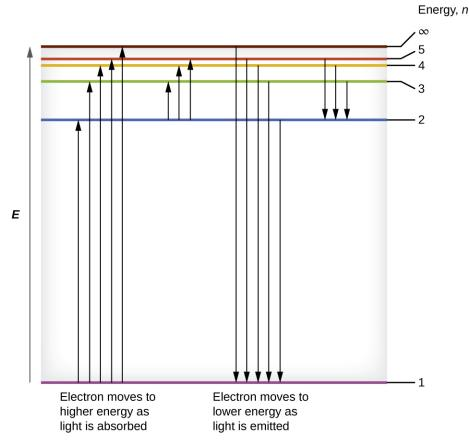
**Figure 3.15** The horizontal lines show the relative energy of orbits in the Bohr model of the hydrogen atom, and the vertical arrows depict the energy of photons absorbed (left) or emitted (right) as electrons move between these orbits.
