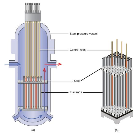
**Figure 20.20** The nuclear reactor core shown in (a) contains the fuel and control rod assembly shown in (b). (credit: modification of work by E. Generalic, http://glossary.periodni.com/glossary.php?en=control+rod)
