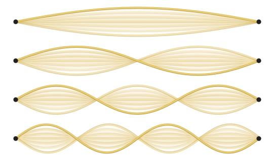
**Figure 3.7** A vibrating string shows some one-dimensional standing waves. Since the two end points of the string are held fixed, only waves having an integer number of half-wavelengths can form. The points on the string between the end points that are not moving are called the nodes.
