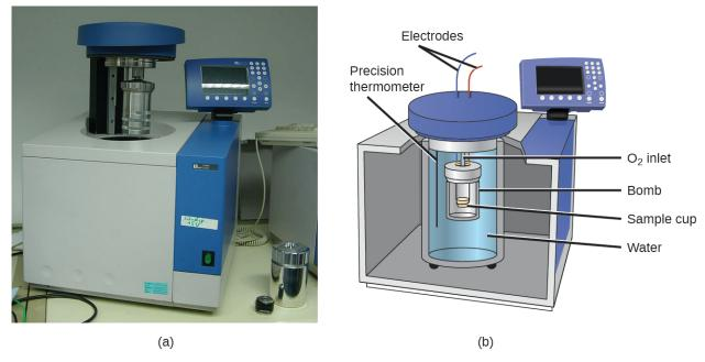
**Figure 9.17** (a) A bomb calorimeter is used to measure heat produced by reactions involving gaseous reactants or products, such as combustion. (b) The reactants are contained in the gas-tight "bomb," which is submerged in water and surrounded by insulating materials. (credit a: modification of work by "Harbor1"/Wikimedia commons)
