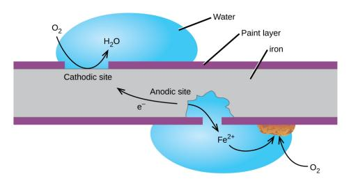
**Figure 16.16** Corrosion can occur when a painted iron or steel surface is exposed to the environment by a scratch through the paint. A galvanic cell results that may be approximated by the simplified cell schematic  $Fe(s) \mid Fe^{2+}(aq) \mid |O_2(aq), H_2O(l)| Fe(s)$ .
