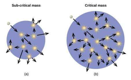
**Figure 20.17** (a) In a subcritical mass, the fissile material is too small and allows too many neutrons to escape the material, so a chain reaction does not occur. (b) In a critical mass, a large enough number of neutrons in the fissile material induce fission to create a chain reaction.
