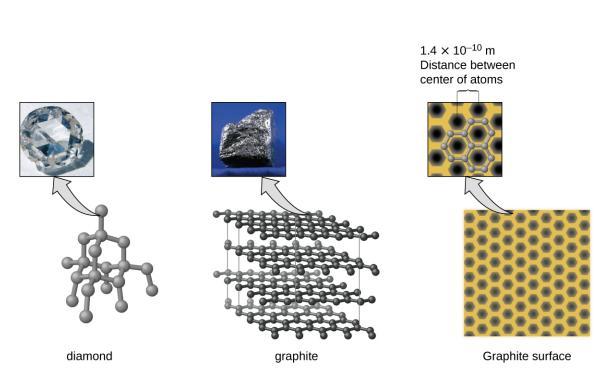
**Figure 10.43** Diamond is extremely hard because of the strong bonding between carbon atoms in all directions. Graphite (in pencil lead) rubs off onto paper due to the weak attractions between the carbon layers. An image of a graphite surface shows the distance between the centers of adjacent carbon atoms. (credit left photo: modification of work by Steve Jurvetson; credit middle photo: modification of work by United States Geological Survey)
