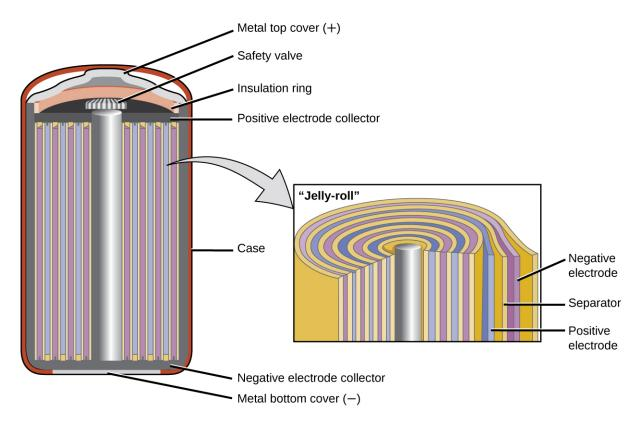
**Figure 16.11** NiCd batteries use a "jelly-roll" design that significantly increases the amount of current the battery can deliver as compared to a similar-sized alkaline battery.
