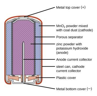
Figure 16.10 Alkaline batteries were designed as improved replacements for zinc-carbon (dry cell) batteries.
