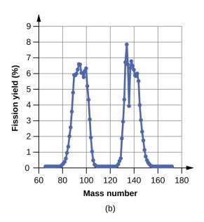
**Figure 20.15** (a) Nuclear fission of U-235 produces a range of fission products. (b) The larger fission products of U-235 are typically one isotope with a mass number around 85–105, and another isotope with a mass number that is about 50% larger, that is, about 130–150.
