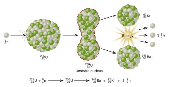
**Figure 20.14** When a slow neutron hits a fissionable U-235 nucleus, it is absorbed and forms an unstable U-236 nucleus. The U-236 nucleus then rapidly breaks apart into two smaller nuclei (in this case, Ba-141 and Kr-92) along with several neutrons (usually two or three), and releases a very large amount of energy.
