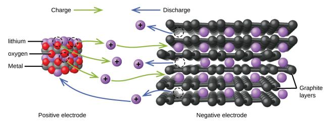
**Figure 16.12** In a lithium ion battery, charge flows as the lithium ions are transferred between the anode and cathode.
