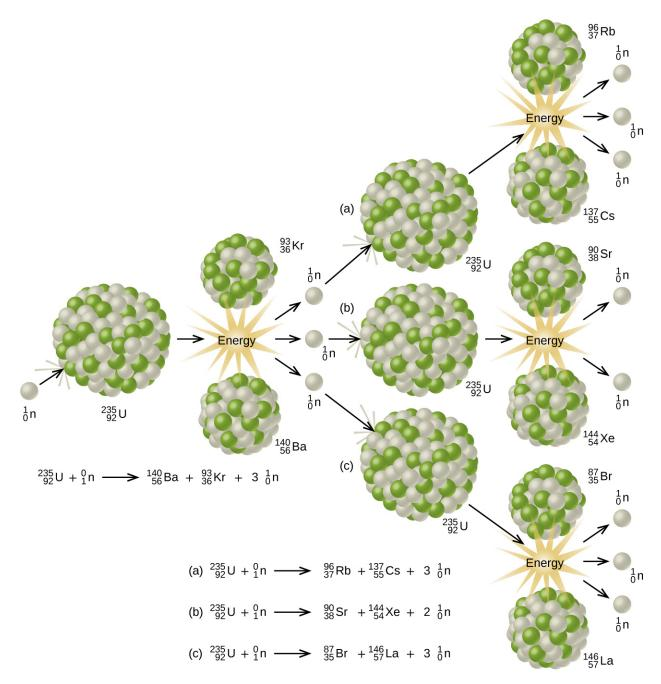
**Figure 20.16** The fission of a large nucleus, such as U-235, produces two or three neutrons, each of which is capable of causing fission of another nucleus by the reactions shown. If this process continues, a nuclear chain reaction occurs.
