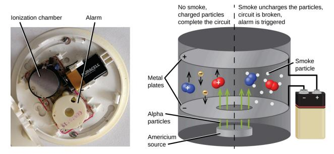
Figure 20.29 Inside a smoke detector, Am-241 emits  $\alpha$  particles that ionize the air, creating a small electric current. During a fire, smoke particles impede the flow of ions, reducing the current and triggering an alarm. (credit a: modification of work by "Muffet"/Wikimedia Commons)
