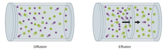
**Figure 8.28** Diffusion involves the unrestricted dispersal of molecules throughout space due to their random motion. When this process is restricted to passage of molecules through very small openings in a physical barrier, the process is called effusion.
