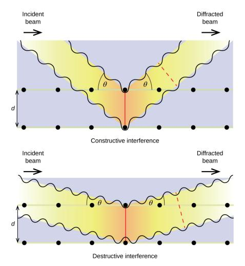
**Figure 10.64** The diffraction of X-rays scattered by the atoms within a crystal permits the determination of the distance between the atoms. The top image depicts constructive interference between two scattered waves and a resultant diffracted wave of high intensity. The bottom image depicts destructive interference and a low intensity diffracted wave.
