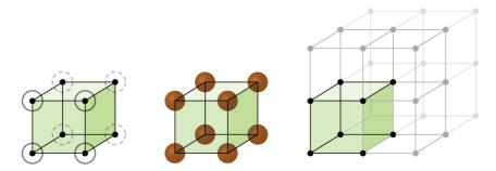
**Figure 10.47** When metal atoms are arranged with spheres in one layer directly above or below spheres in another layer, the lattice structure is called simple cubic. Note that the spheres are in contact.
