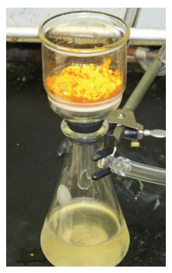
Figure 7.17 Precipitate may be removed from a reaction mixture by filtration.
