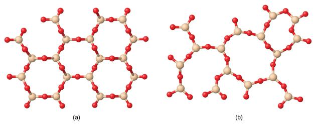
**Figure 10.38** (a) Silicon dioxide, SiO<sub>2</sub>, is abundant in nature as one of several crystalline forms of the mineral quartz. (b) Rapid cooling of molten SiO<sub>2</sub> yields an amorphous solid known as "fused silica".
