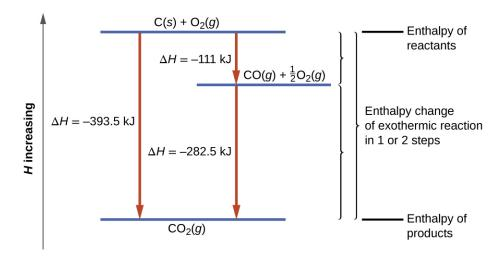
**Figure 9.24** The formation of  $CO_2(g)$  from its elements can be thought of as occurring in two steps, which sum to the overall reaction, as described by Hess's law. The horizontal blue lines represent enthalpies. For an exothermic process, the products are at lower enthalpy than are the reactants.
