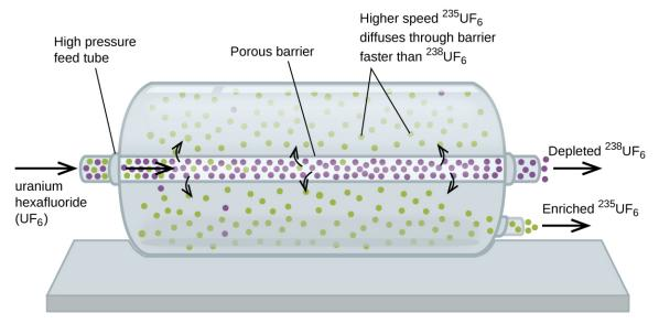
**Figure 8.30** In a diffuser, gaseous UF<sub>6</sub> is pumped through a porous barrier, which partially separates  $^{235}$ UF<sub>6</sub> from  $^{238}$ UF<sub>6</sub> The UF<sub>6</sub> must pass through many large diffuser units to achieve sufficient enrichment in  $^{235}$ U.
