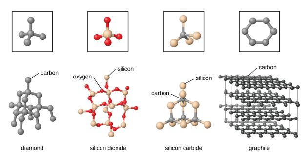
**Figure 10.41** A covalent crystal contains a three-dimensional network of covalent bonds, as illustrated by the structures of diamond, silicon dioxide, silicon carbide, and graphite. Graphite is an exceptional example, composed of planar sheets of covalent crystals that are held together in layers by noncovalent forces. Unlike typical covalent solids, graphite is very soft and electrically conductive.
