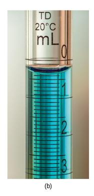
**Figure 7.16** (a) A student fills a buret in preparation for a titration analysis. (b) A typical buret permits volume measurements to the nearest 0.01 mL. (credit a: modification of work by Mark Blaser and Matt Evans; credit b: modification of work by Mark Blaser and Matt Evans)
