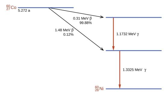
Figure 20.27 Co-60 undergoes a series of radioactive decays. The y emissions are used for radiation therapy.
