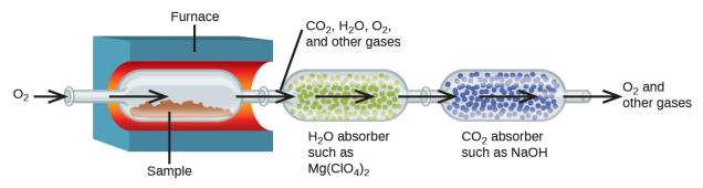
**Figure 7.18** This schematic diagram illustrates the basic components of a combustion analysis device for determining the carbon and hydrogen content of a sample.
