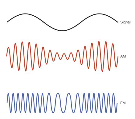
Figure 3.5 This schematic depicts how amplitude modulation (AM) and frequency modulation (FM) can be used to transmit a radio wave.
