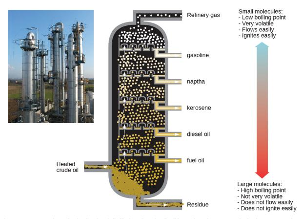
**Figure 21.6** In a column for the fractional distillation of crude oil, oil heated to about 425 °C in the furnace vaporizes when it enters the base of the tower. The vapors rise through bubble caps in a series of trays in the tower. As the vapors gradually cool, fractions of higher, then of lower, boiling points condense to liquids and are drawn off. (credit left: modification of work by Luigi Chiesa)
