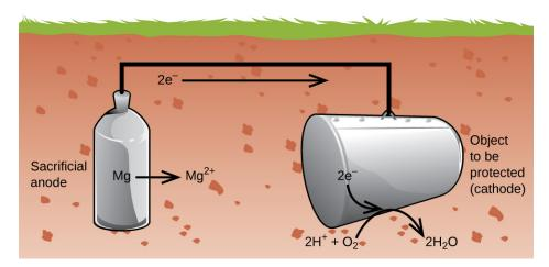
**Figure 16.17** Cathodic protection is a useful approach to electrochemically preventing corrosion of underground storage tanks.
