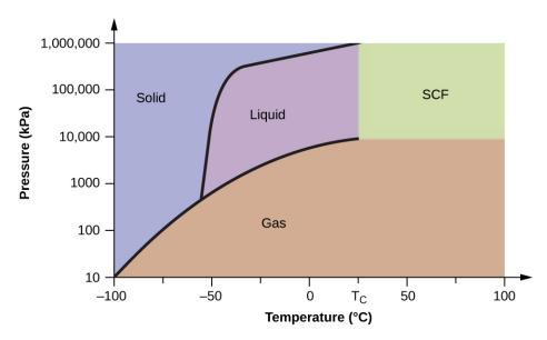
**Figure 10.34** A phase diagram for carbon dioxide is shown. The pressure axis is plotted on a logarithmic scale to accommodate the large range of values.
