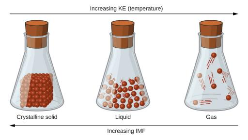
**Figure 10.2** Transitions between solid, liquid, and gaseous states of a substance occur when conditions of temperature or pressure favor the associated changes in intermolecular forces. (Note: The space between particles in the gas phase is much greater than shown.)
