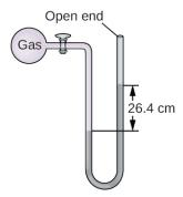
**17.** How would the use of a volatile liquid affect the measurement of a gas using open-ended manometers vs. closed-end manometers?
