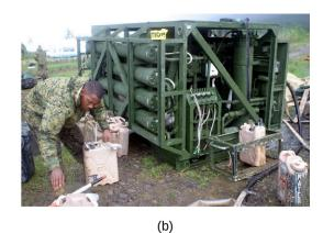
**Figure 11.26** Reverse osmosis systems for purifying drinking water are shown here on (a) small and (b) large scales. (credit a: modification of work by Jerry Kirkhart; credit b: modification of work by Willard J. Lathrop)
