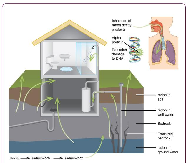
**Figure 20.34** Radon-222 seeps into houses and other buildings from rocks that contain uranium-238, a radon emitter. The radon enters through cracks in concrete foundations and basement floors, stone or porous cinderblock foundations, and openings for water and gas pipes.
