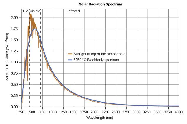
**Figure 3.9** The spectral distribution (light intensity vs. wavelength) of sunlight reaches the Earth's atmosphere as UV light, visible light, and IR light. The unabsorbed sunlight at the top of the atmosphere has a distribution that approximately matches the theoretical distribution of a blackbody at 5250 °C, represented by the blue curve. (credit: modification of work by American Society for Testing and Materials (ASTM) Terrestrial Reference Spectra for Photovoltaic Performance Evaluation)
