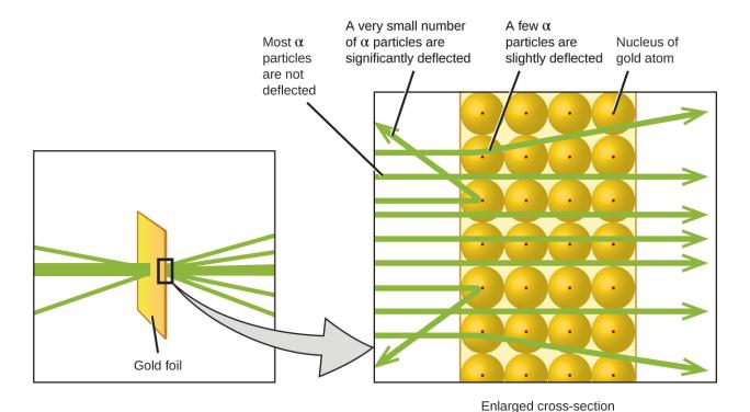
Figure 2.10 The  $\alpha$  particles are deflected only when they collide with or pass close to the much heavier, positively charged gold nucleus. Because the nucleus is very small compared to the size of an atom, very few  $\alpha$  particles are deflected. Most pass through the relatively large region occupied by electrons, which are too light to deflect the rapidly moving particles.
