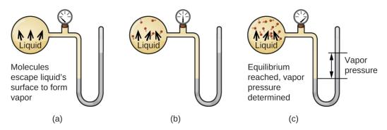
**Figure 10.22** In a closed container, dynamic equilibrium is reached when (a) the rate of molecules escaping from the liquid to become the gas (b) increases and eventually (c) equals the rate of gas molecules entering the liquid. When this equilibrium is reached, the vapor pressure of the gas is constant, although the vaporization and condensation processes continue.
