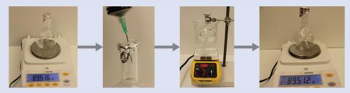
**Figure 8.19** When the volatile liquid in the flask is heated past its boiling point, it becomes gas and drives air out of the flask. At  $t_l \longrightarrow g$ , the flask is filled with volatile liquid gas at the same pressure as the atmosphere. If the flask is then cooled to room temperature, the gas condenses and the mass of the gas that filled the flask, and is now liquid, can be measured. (credit: modification of work by Mark Ott)
