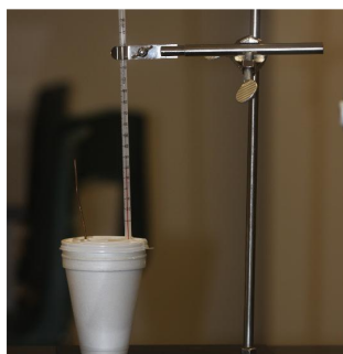
Figure 15: (Left panel) A coffee-cup calorimeter. (Right panel) A constant-volume calorimeter.
