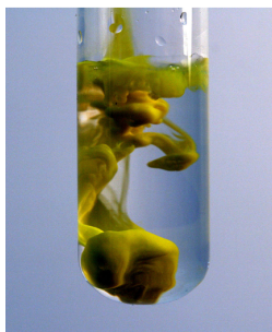
Figure 12: (Left panel) A precipitate of \text{PbI}_2 ; (Right panel) The result of an acid-base neutralization.
