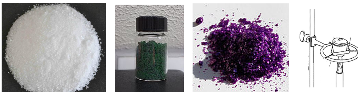
Figure 11: Several chemical hydrates used in this experiment: (Left panel) \text{CaCl}_2 \cdot 6\text{H}_2\text{O} ; (Central left panel) \text{CrCl}_3 \cdot 6\text{H}_2\text{O} ; (Central right panel) anhydrous \text{CrCl}_3 ; (Right Panel) The set up for the experiment.
