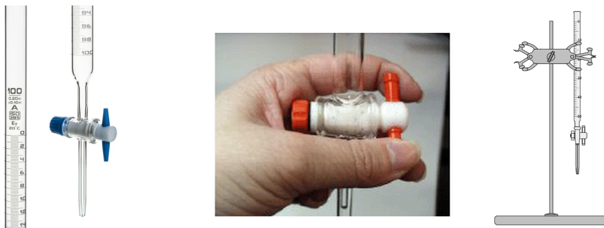
Figure 13: (Left panel) A buret employed in a titration. (Center panel) Illustration showing the correct way to control the buret valve. (Right panel) The titration set up
