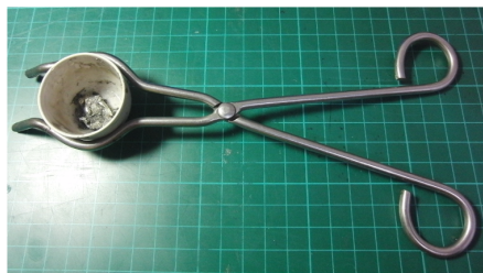
Figure 7: (Left panel) A crucible. (Central panel) Use of the crucible tongs. (Right panel) Correct arrangement of the ring stand.
