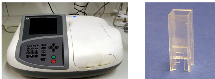
Figure 8: (Left panel) A spectrophotometer. (Right panel) A cuvette.
