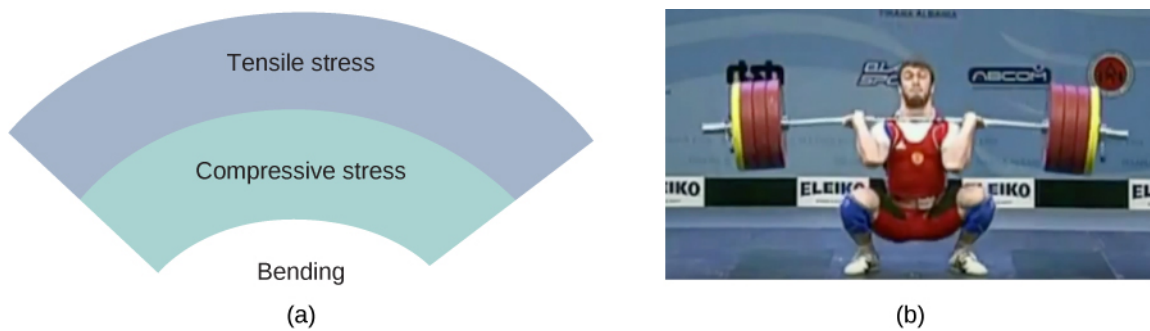
Figure 12.20 (a) An object bending downward experiences tensile stress (stretching) in the upper section and compressive stress (compressing) in the lower section. (b) Elite weightlifters often bend iron bars temporarily during lifting, as in the 2012 Olympics competition. (credit b: modification of work by Oleksandr Kocherzhenko)
