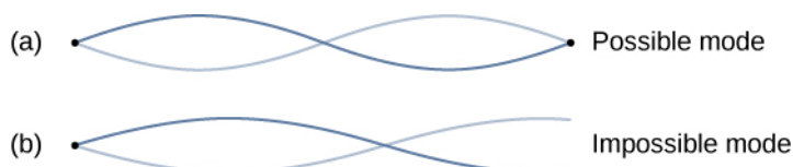
Figure 16.31 (a) The figure represents the second mode of the string that satisfies the boundary conditions of a node at each end of the string. (b) This figure could not possibly be a normal mode on the string because it does not satisfy the boundary conditions. There is a node on one end, but an antinode on the other.
