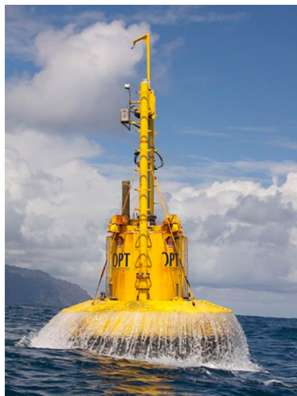
Figure 16.1 From the world of renewable energy sources comes the electric power-generating buoy. Although there are many versions, this one converts the up-and-down motion, as well as side-to-side motion, of the buoy into rotational motion in order to turn an electric generator, which stores the energy in batteries.
