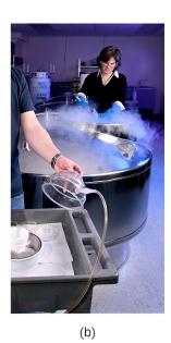
Figure 13.10 Cultures and other medical specimens can be stored for long periods at ultra-low temperatures. (a) An ultra-low freezer maintains temperatures at or below –70 °C. (b) Even lower temperatures can be achieved through freezing and storage in liquid nitrogen. (credit a: modification of work by "Expert Infantry"/Flickr; credit b: modification of work by USDA)
