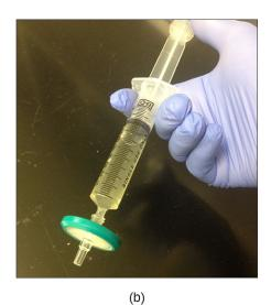
**Figure 13.16** Membrane filters come in a variety of sizes, depending on the volume of solution being filtered. (a) Larger volumes are filtered in units like these. The solution is drawn through the filter by connecting the unit to a vacuum. (b) Smaller volumes are often filtered using syringe filters, which are units that fit on the end of a syringe. In this case, the solution is pushed through by depressing the syringe's plunger. (credit a, b: modification of work by Brian Forster)
