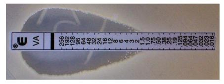
Figure 14.21 The Etest can be used to determine the MIC of an antibiotic. In this Etest, vancomycin is shown to have a MIC of 1.5 μg/mL against *Staphylococcus aureus*.
