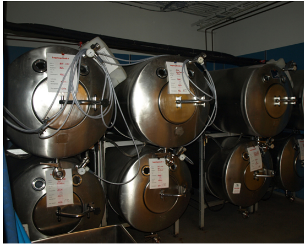
Figure 4.18 Fermentation of grape juice to make wine produces CO 2 as a byproduct. Fermentation tanks have valves so that pressure inside the tanks can be released.
