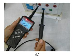
Figure 21.27 (a) To measure potential differences in this series circuit, the voltmeter (V) is placed in parallel with the voltage source or either of the resistors. Note that terminal voltage is measured between points a and b. It is not possible to connect the voltmeter directly across the emf without including its internal resistance, r. (b) A digital voltmeter in use. (credit: Messtechniker, Wikimedia Commons)
