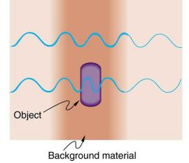
Figure 27.51 Light rays passing through a sample under a microscope will emerge with different phases depending on their paths. The object shown has a greater index of refraction than the background, and so the wavelength decreases as the ray passes through it. Superimposing these rays produces interference that varies with path, enhancing contrast between the object and background.
