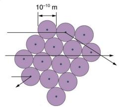
Figure 30.11 An expanded view of the atoms in the gold foil in Rutherford's experiment. Circles represent the atoms (about  $10^{-10}$  m in diameter),
