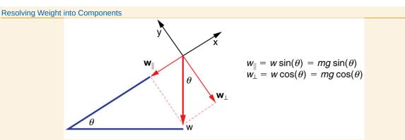
**Figure 4.14** An object rests on an incline that makes an angle  $\theta$  with the horizontal.
