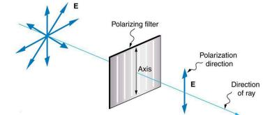
Figure 27.40 A polarizing filter has a polarization axis that acts as a slit passing through electric fields parallel to its direction. The direction of polarization of an EM wave is defined to be the direction of its electric field.
