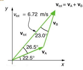
Figure 3.55 The two velocities  $\,v_A\,$  and  $\,v_B\,$  add to give a total  $\,v_{tot}\,$  .
