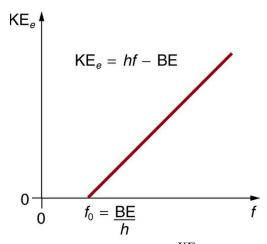
Figure 29.9 Photoelectric effect. A graph of the kinetic energy of an ejected electron,  $KE_e$ , versus the frequency of EM radiation impinging on a certain material. There is a threshold frequency below which no electrons are ejected, because the individual photon interacting with an individual electron has insufficient energy to break it away. Above the threshold energy,  $KE_e$  increases linearly with f, consistent with  $KE_e = hf - BE$ .
