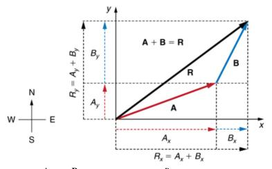
Figure 3.32 The magnitude of the vectors  $\mathbf{A}_x$  and  $\mathbf{B}_x$  add to give the magnitude  $R_x$  of the resultant vector in the horizontal direction. Similarly, the magnitudes of the vectors  $\mathbf{A}_y$  and  $\mathbf{B}_y$  add to give the magnitude  $R_y$  of the resultant vector in the vertical direction.
