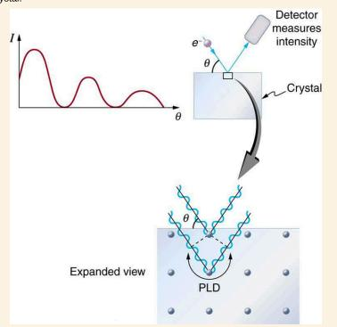
Figure 29.23 The diffraction pattern at top left is produced by scattering electrons from a crystal and is graphed as a function of incident angle relative to the regular array of atoms in a crystal, as shown at bottom. Electrons scattering from the second layer of atoms travel farther than those scattered from the top layer. If the path length difference (PLD) is an integral wavelength, there is constructive interference.
