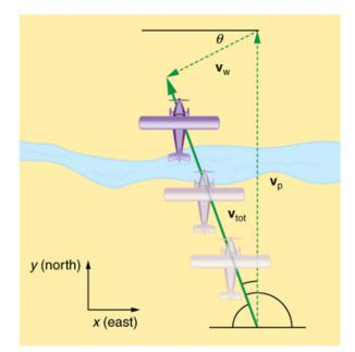
Figure 3.44 An airplane heading straight north is instead carried to the west and slowed down by wind. The plane does not move relative to the ground in the direction it points; rather, it moves in the direction of its total velocity (solid arrow).
