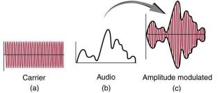
Figure 24.12 Amplitude modulation for AM radio. (a) A carrier wave at the station's basic frequency. (b) An audio signal at much lower audible frequencies. (c) The amplitude of the carrier is modulated by the audio signal without changing its basic frequency.
