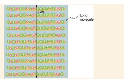
Figure 27.44 Long molecules are aligned perpendicular to the axis of a polarizing filter. The component of the electric field in an EM wave perpendicular to these molecules passes through the filter, while the component parallel to the molecules is absorbed.
