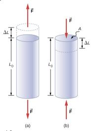
Figure 5.13 (a) Tension. The rod is stretched a length  $\Delta L$  when a force is applied parallel to its length. (b) Compression. The same rod is compressed by forces with the same magnitude in the opposite direction. For very small deformations and uniform materials,  $\Delta L$  is approximately the same for the same magnitude of tension or compression. For larger deformations, the cross-sectional area changes as the rod is compressed or stretched.
