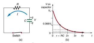
Figure 21.39 (a) Closing the switch discharges the capacitor C through the resistor R. Mutual repulsion of like charges on each plate drives the current. (b) A graph of voltage across the capacitor versus time, with  $V = V_0$  at t = 0. The voltage decreases exponentially, falling a fixed fraction of the way to zero in each subsequent time constant  $\tau$ .
