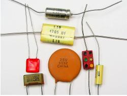
Figure 19.15 Some typical capacitors. Size and value of capacitance are not necessarily related. (credit: Windell Oskay)
