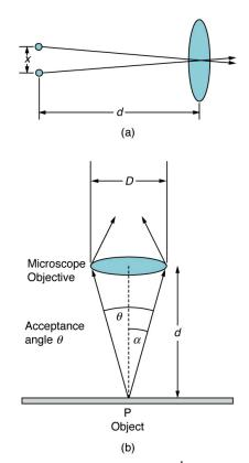
Figure 27.30 (a) Two points separated by at distance x and a positioned a distance d away from the objective. (credit: Infopro, Wikimedia Commons) (b) Terms and symbols used in discussion of resolving power for a lens and an object at point P. (credit: Infopro, Wikimedia Commons)
