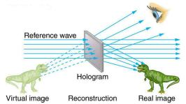
Figure 30.45 A transmission hologram is one that produces real and virtual images when a laser of the same type as that which exposed the hologram is passed through it. Diffraction from various parts of the film produces the same interference pattern as the object that was used to expose it.
