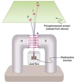
Figure 31.3 Alpha, beta, and gamma rays are passed through a magnetic field on the way to a phosphorescent screen. The  $\alpha$  s and  $\beta$  s bend in opposite directions, while the  $\gamma$  s are unaffected, indicating a positive charge for  $\alpha$  s, negative for  $\beta$  s, and neutral for  $\gamma$  s. Consistent results are obtained with electric fields. Collection of the radiation offers further confirmation from the direct measurement of excess charge.
