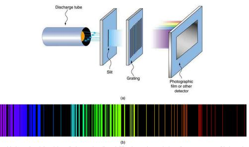
Figure 30.15 Part (a) shows, from left to right, a discharge tube, slit, and diffraction grating producing a line spectrum. Part (b) shows the emission line spectrum for iron. The discrete lines imply quantized energy states for the atoms that produce them. The line spectrum for each element is unique, providing a powerful and much used analytical tool, and many line spectra were well known for many years before they could be explained with physics. (credit for (b): Yttrium91, Wikimedia Commons)
