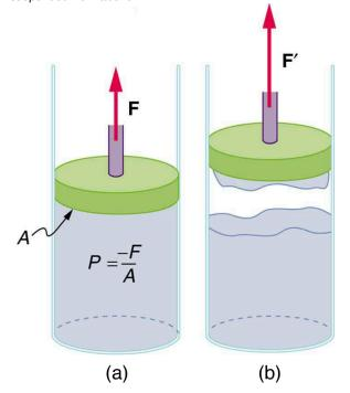
**Figure 11.43** (a) When the piston is raised, it stretches the liquid slightly, putting it under tension and creating a negative absolute pressure P = -F/A (b) The liquid eventually separates, giving an experimental limit to negative pressure in this liquid.
