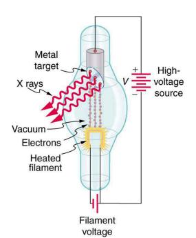
Figure 29.13 X rays are produced when energetic electrons strike the copper anode of this cathode ray tube (CRT). Electrons (shown here as separate particles) interact individually with the material they strike, sometimes producing photons of EM radiation.
