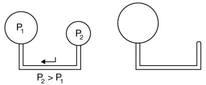
Figure 11.29 With the valve closed, two balloons of different sizes are attached to each end of a tube. Upon opening the valve, the smaller balloon decreases in size with the air moving to fill the larger balloon. The pressure in a spherical balloon is inversely proportional to its radius, so that the smaller balloon has a greater internal pressure than the larger balloon, resulting in this flow.
