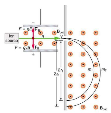
Figure 22.43 This mass spectrometer uses a velocity selector to fix v so that the radius of the path is proportional to mass.
