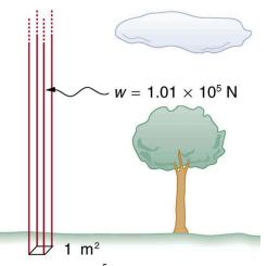
Figure 11.11 Atmospheric pressure at sea level averages  $1.01 \times 10^5$  Pa (equivalent to 1 atm), since the column of air over this  $1 \text{ m}^2$ , extending to the top of the atmosphere, weighs  $1.01 \times 10^5$  N.
