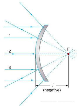
Figure 25.42 Parallel rays of light reflected from a convex spherical mirror (small in size compared with its radius of curvature) seem to originate from a well-defined focal point at the focal distance f behind the mirror. Convex mirrors diverge light rays and, thus, have a negative focal length.
