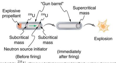
Figure 32.27 A gun-type fission bomb for  $^{235}$  U utilizes two subcritical masses forced together by explosive charges inside a cannon barrel. The energy yield depends on the amount of uranium and the time it can be held together before it disassembles itself.
