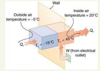
Figure 15.30 Heat transfer from the outside to the inside, along with work done to run the pump, takes place in the heat pump of the example above. Note that the cold temperature produced by the heat pump is lower than the outside temperature, so that heat transfer into the working fluid occurs. The pump's compressor produces a temperature greater than the indoor temperature in order for heat transfer into the house to occur.
