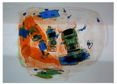
Figure 30.26 This x-ray image shows the contents of a piece of luggage. The denser the material, the darker the shadow. (credit: IDuke, Wikimedia Commons)
