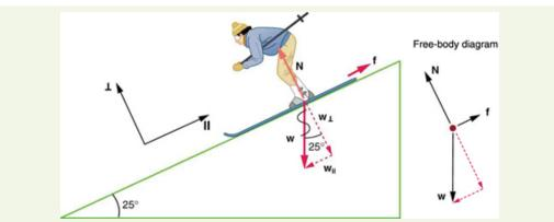
Figure 4.13 Since motion and friction are parallel to the slope, it is most convenient to project all forces onto a coordinate system where one axis is parallel to the slope and the other is perpendicular (axes shown to left of skier). N is perpendicular to the slope and f is parallel to the slope, but w has components along both axes, namely  $w_{\perp}$  and  $w_{\parallel}$ . N is equal in magnitude to  $w_{\perp}$ , so that there is no motion
