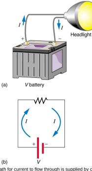
Figure 20.3 (a) A simple electric circuit. A closed path for current to flow through is supplied by conducting wires connecting a load to the terminals of a battery. (b) In this schematic, the battery is represented by the two parallel red lines, conducting wires are shown as straight lines, and the zigzag represents the load. The schematic represents a wide variety of similar circuits.
