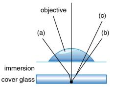
Figure 26.19 Light rays from a specimen entering the objective. Paths for immersion medium of air (a), water (b) (n = 1.33), and oil (c)
