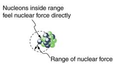
Figure 31.27 The nuclear force is attractive and stronger than the Coulomb force, but it is short ranged. In low-mass nuclei, each nucleon feels the nuclear attraction of all others. In larger nuclei, the range of the nuclear force, shown for a single nucleon, is smaller than the size of the nucleus, but the Coulomb repulsion from all protons reaches all others. If the nucleus is large enough, the Coulomb repulsion can add to overcome the nuclear attraction.
