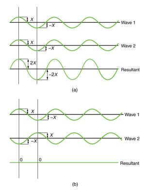
Figure 27.11 The amplitudes of waves add. (a) Pure constructive interference is obtained when identical waves are in phase. (b) Pure destructive interference occurs when identical waves are exactly out of phase, or shifted by half a wavelength.
