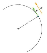
Figure 10.4 In circular motion, linear acceleration a, occurs as the magnitude of the velocity changes: a is tangent to the motion. In the context of circular motion, linear acceleration is also called tangential acceleration  $a_{t}$ .
