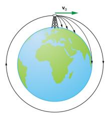
Figure 3.41 Projectile to satellite. In each case shown here, a projectile is launched from a very high tower to avoid air resistance. With increasing initial speed, the range increases and becomes longer than it would be on level ground because the Earth curves away underneath its path. With a large enough initial speed, orbit is achieved.
