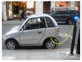
Figure 20.44 This REVAi, an electric car, gets recharged on a street in London. (credit: Frank Hebbert)
