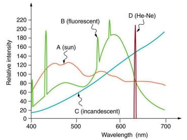
Figure 26.12 Emission spectra for various light sources are shown. Curve A is average sunlight at Earth's surface, curve B is light from a fluorescent lamp, and curve C is the output of an incandescent light. The spike for a helium-neon laser (curve D) is due to its pure wavelength emission. The spikes in the fluorescent output are due to atomic spectra—a topic that will be explored later.
