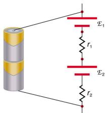
Figure 21.15 A series connection of two voltage sources. The emfs (each labeled with a script E) and internal resistances add, giving a total emf of  $emf_1 + emf_2$  and a total internal resistance of  $r_1 + r_2$ .
