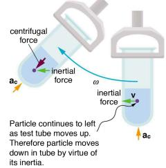
Figure 6.17 Centrifuges use inertia to perform their task. Particles in the fluid sediment come out because their inertia carries them away from the center of rotation. The large angular velocity of the centrifuge quickens the sedimentation. Ultimately, the particles will come into contact with the test tube walls, which will then supply the centripetal force needed to make them move in a circle of constant radius.
