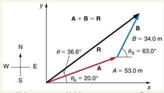
Figure 3.33 Vector  $\mathbf{A}$  has magnitude 53.0 m and direction 20.0 ° north of the *x*-axis. Vector  $\mathbf{B}$  has magnitude 34.0 m and direction 63.0° north of the *x*-axis. You can use analytical methods to determine the magnitude and direction of  $\mathbf{R}$ .
