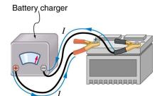
Figure 21.14 A car battery charger reverses the normal direction of current through a battery, reversing its chemical reaction and replenishing its chemical potential.
