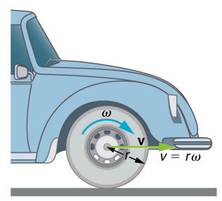
Figure 6.5 A car moving at a velocity v to the right has a tire rotating with an angular velocity  $\omega$ . The speed of the tread of the tire relative to the axle is v, the same as if the car were jacked up. Thus the car moves forward at linear velocity  $v = r\omega$ , where r is the tire radius. A larger angular velocity for the tire means a greater velocity for the car.
