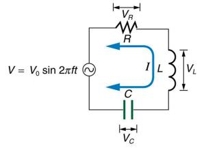
Figure 23.48 An RLC series circuit with an AC voltage source.
