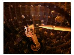
Figure 30.41 This system of lasers at Lawrence Livermore Laboratory is used to ignite nuclear fusion. A tremendous burst of energy is focused on a small fuel pellet, which is imploded to the high density and temperature needed to make the fusion reaction proceed. (credit: Lawrence Livermore National Laboratory, Lawrence Livermore National Security, LLC, and the Department of Energy)
