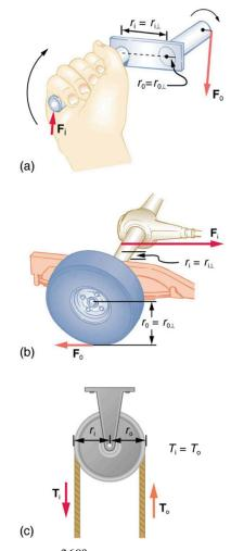
**Figure 9.24** (a) A crank is a type of lever that can be rotated  $360^{\circ}$  about its pivot. Cranks are usually designed to have a large MA. (b) A simplified automobile axle drives a wheel, which has a much larger diameter than the axle. The MA is less than 1. (c) An ordinary pulley is used to lift a heavy load. The pulley changes the direction of the force T exerted by the cord without changing its magnitude. Hence, this machine has an MA of 1.
