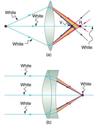
Figure 26.28 (a) Chromatic aberration is caused by the dependence of a lens's index of refraction on color (wavelength). The lens is more powerful for violet (V) than for red (R), producing images with different locations and magnifications. (b) Multiple-lens systems can partially correct chromatic aberrations, but they may require lenses of different materials and add to the expense of optical systems such as cameras.
