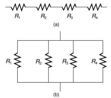
Figure 21.2 (a) A series connection of resistors. (b) A parallel connection of resistors.
