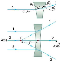
Figure 25.29 Rays of light entering a diverging lens parallel to its axis are diverged, and all appear to originate at its focal point F. The dashed lines are not rays—they indicate the directions from which the rays appear to come. The focal length f of a diverging lens is negative. An expanded view of the path taken by ray 1 shows the perpendiculars and the angles of incidence and refraction at both surfaces.
