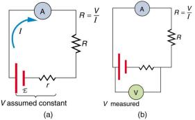
Figure 21.36 Two methods for measuring resistance with standard meters. (a) Assuming a known voltage for the source, an ammeter measures current, and resistance is calculated as  $R = \frac{V}{I}$ . (b) Since the terminal voltage V varies with current, it is better to measure it. V is most accurately known when I is small, but I itself is most accurately known when it is large.
