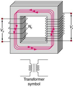
Figure 23.28 A typical construction of a simple transformer has two coils wound on a ferromagnetic core that is laminated to minimize eddy currents. The magnetic field created by the primary is mostly confined to and increased by the core, which transmits it to the secondary coil. Any change in current in the primary induces a current in the secondary.
