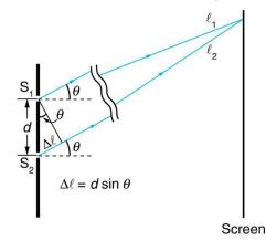
Figure 27.14 The paths from each slit to a common point on the screen differ by an amount  $d \sin \theta$ , assuming the distance to the screen is much greater than the distance between slits (not to scale here).
