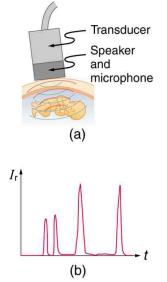
Figure 17.43 (a) An ultrasound speaker doubles as a microphone. Brief bleeps are broadcast, and echoes are recorded from various depths. (b) Graph of echo intensity versus time. The time for echoes to return is directly proportional to the distance of the reflector, yielding this information noninvasively.
