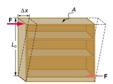
Figure 5.16 Shearing forces are applied perpendicular to the length  $L_0$  and parallel to the area A, producing a deformation  $\Delta x$ . Vertical forces
