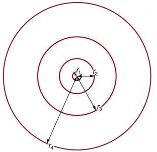
Figure 30.19 The allowed electron orbits in hydrogen have the radii shown. These radii were first calculated by Bohr and are given by the equation  $r_n = \frac{n^2}{Z} a_B$ . The lowest orbit has the experimentally verified diameter of a hydrogen atom.
