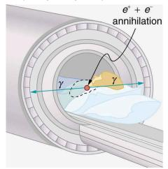
Figure 32.7 A PET system takes advantage of the two identical  $\gamma$ -ray photons produced by positron-electron annihilation. These  $\gamma$  rays are emitted in opposite directions, so that the line along which each pair is emitted is determined. Various events detected by several pairs of detectors are then analyzed by the computer to form an accurate image.
