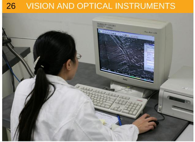
Figure 26.1 A scientist examines minute details on the surface of a disk drive at a magnification of 100,000 times. The image was produced using an electron microscope. (credit: Robert Scoble)
