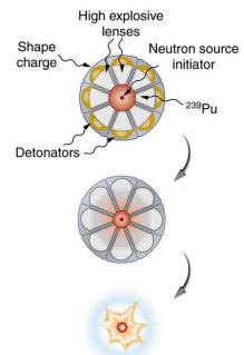
Figure 32.28 An implosion created by high explosives compresses a sphere of  $^{239}$ Pu into a critical mass. The superior fissionability of plutonium has made it the universal bomb material.
