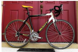
Figure 10.32 The image shows a side view of a racing bicycle. Can you see evidence in the design of the wheels on this racing bicycle that their moment of inertia has been purposely reduced? (credit: Jesús Rodriguez)
