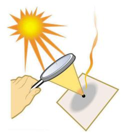
Figure 25.28 Sunlight focused by a converging magnifying glass can burn paper. Light rays from the sun are nearly parallel and cross at the focal point of the lens. The more powerful the lens, the closer to the lens the rays will cross.
