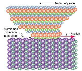
Figure 5.6 The tip of a probe is deformed sideways by frictional force as the probe is dragged across a surface. Measurements of how the force varies for different materials are yielding fundamental insights into the atomic nature of friction.
