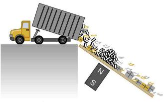
Figure 23.17 Metals can be separated from other trash by magnetic drag. Eddy currents and magnetic drag are created in the metals sent down this ramp by the powerful magnet beneath it. Nonmetals move on.
