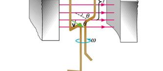
Figure 23.21 A generator with a single rectangular coil rotated at constant angular velocity in a uniform magnetic field produces an emf that varies sinusoidally in time. Note the generator is similar to a motor, except the shaft is rotated to produce a current rather than the other way around.
