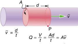
Figure 12.2 Flow rate is the volume of fluid per unit time flowing past a point through the area A. Here the shaded cylinder of fluid flows past point P in a uniform pipe in time t. The volume of the cylinder is Ad and the average velocity is v = d/t so that the flow rate is Q = Ad/t = Av.
