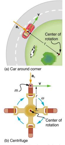
Figure 6.9 (a) The car following a circular path at constant speed is accelerated perpendicular to its velocity, as shown. The magnitude of this centripetal acceleration is found in Example 6.2. (b) A particle of mass in a centrifuge is rotating at constant angular velocity. It must be accelerated perpendicular to its velocity or it would continue in a straight line. The magnitude of the necessary acceleration is found in Example 6.3.
