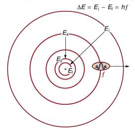
Figure 30.17 The planetary model of the atom, as modified by Bohr, has the orbits of the electrons quantized. Only certain orbits are allowed, explaining why atomic spectra are discrete (quantized). The energy carried away from an atom by a photon comes from the electron dropping from one allowed orbit to another and is thus quantized. This is likewise true for atomic absorption of photons.
