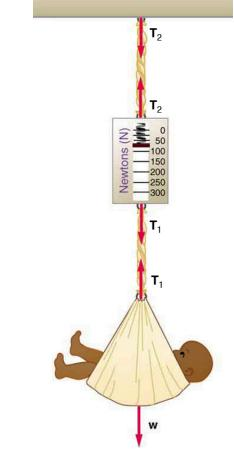
Figure 4.33 A baby is weighed using a spring scale.
