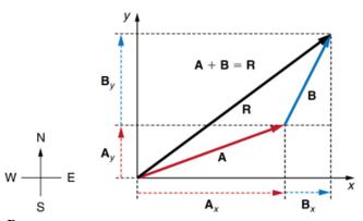
Figure 3.31 To add vectors  $\bf{A}$  and  $\bf{B}$ , first determine the horizontal and vertical components of each vector. These are the dotted vectors  $\bf{A}_{\chi}$ ,
