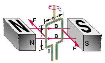
Figure 22.34 Torque on a current loop. A current-carrying loop of wire attached to a vertically rotating shaft feels magnetic forces that produce a clockwise torque as viewed from above.
