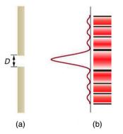
Figure 27.21 (a) Single slit diffraction pattern. Monochromatic light passing through a single slit has a central maximum and many smaller and dimmer maxima on either side. The central maximum is six times higher than shown. (b) The drawing shows the bright central maximum and dimmer and thinner maxima on either side.
