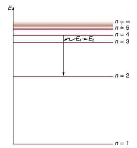
Figure 30.18 An energy-level diagram plots energy vertically and is useful in visualizing the energy states of a system and the transitions between them. This diagram is for the hydrogen-atom electrons, showing a transition between two orbits having energies  $E_4$  and  $E_2$ .
