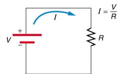
Figure 20.8 A simple electric circuit in which a closed path for current to flow is supplied by conductors (usually metal wires) connecting a load to the terminals of a battery, represented by the red parallel lines. The zigzag symbol represents the single resistor and includes any resistance in the connections to the voltage source.
