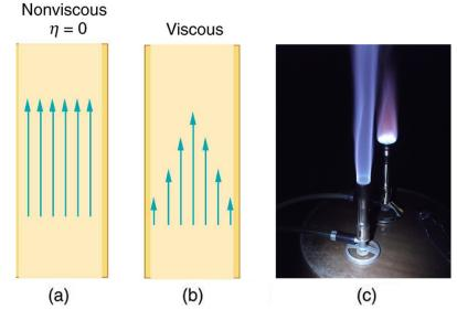
Figure 12.13 (a) If fluid flow in a tube has negligible resistance, the speed is the same all across the tube. (b) When a viscous fluid flows through a tube, its speed at the walls is zero, increasing steadily to its maximum at the center of the tube. (c) The shape of the Bunsen burner flame is due to the velocity profile across the tube. (credit: Jason Woodhead)
