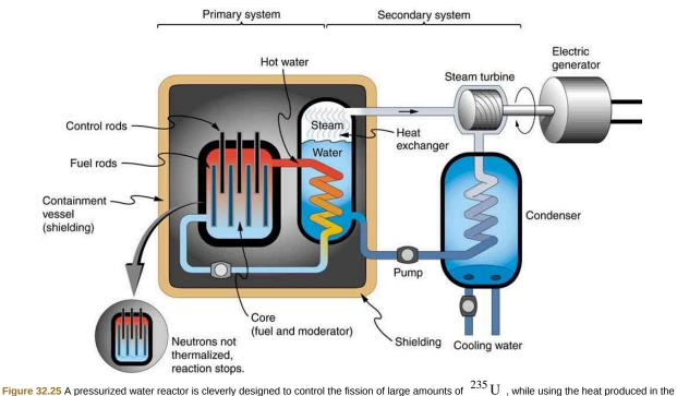
fission reaction to create steam for generating electrical energy. Control rods adjust neutron flux so that criticality is obtained, but not exceeded. In case the reactor overheats and boils the water away, the chain reaction terminates, because water is needed to thermalize the neutrons. This inherent safety feature can be overwhelmed in extreme circumstances.
