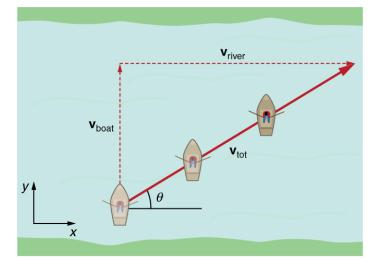
Figure 3.43 A boat trying to head straight across a river will actually move diagonally relative to the shore as shown. Its total velocity (solid arrow) relative to the shore is the sum of its velocity relative to the river plus the velocity of the river relative to the shore.
