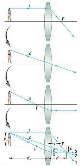
Figure 25.33 Ray tracing is used to locate the image formed by a lens. Rays originating from the same point on the object are traced—the three chosen rays each follow one of the rules for ray tracing, so that their paths are easy to determine. The image is located at the point where the rays cross. In this case, a real image—one that can be projected on a screen—is formed.
