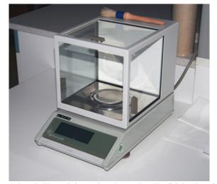
Figure 1.23 Many mechanical balances, such as double-pan balances, have been replaced by digital scales, which can typically measure the mass of an object more precisely. Whereas a mechanical balance may only read the mass of an object to the nearest tenth of a gram, many digital scales can measure the mass of an object up to the nearest thousandth of a gram. (credit: Karel Jakubec)
