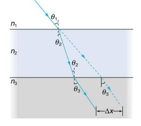
Figure 25.54 A ray of light passes from one medium to a third by traveling through a second. The final direction is the same as if the second medium were not present, but the ray is displaced by  $\Delta x$  (shown exaggerated).
