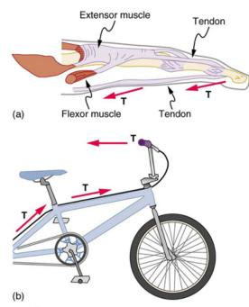
Figure 4.16 (a) Tendons in the finger carry force T from the muscles to other parts of the finger, usually changing the force's direction, but not its magnitude (the tendons are relatively friction free). (b) The brake cable on a bicycle carries the tension T from the handlebars to the brake mechanism. Again, the direction but not the magnitude of T is changed.
