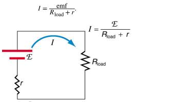
Figure 21.12 Schematic of a voltage source and its load  $R_{load}$ . Since the internal resistance r is in series with the load, it can significantly affect the terminal voltage and current delivered to the load. (Note that the script E stands for emf.)
