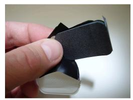
Figure 31.8 Film badges contain film similar to that used in this dental x-ray film and is sandwiched between various absorbers to determine the penetrating ability of the radiation as well as the amount. (credit: Werneuchen, Wikimedia Commons)
