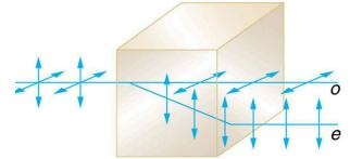
Figure 27.50 Birefringent materials, such as the common mineral calcite, split unpolarized beams of light into two. The ordinary ray behaves as expected, but the extraordinary ray does not obey Snell's law.
