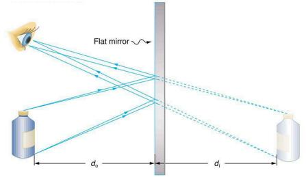
Figure 25.40 Two sets of rays from common points on an object are reflected by a flat mirror into the eye of an observer. The reflected rays seem to originate from behind the mirror, locating the virtual image.
