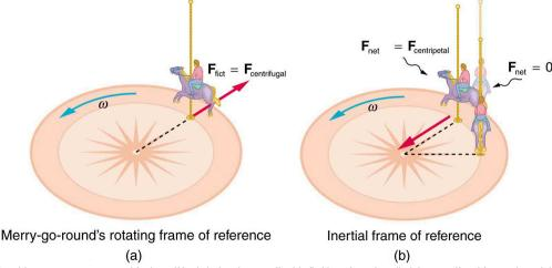
**Figure 6.16** (a) A rider on a merry-go-round feels as if he is being thrown off. This fictitious force is called the centrifugal force—it explains the rider's motion in the rotating frame of reference. (b) In an inertial frame of reference and according to Newton's laws, it is his inertia that carries him off and not a real force (the unshaded rider has  $F_{\text{net}} = 0$  and heads in a straight line). A real force,  $F_{\text{centripetal}}$ , is needed to cause a circular path.
