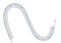
Figure 25.14 Light entering a thin fiber may strike the inside surface at large or grazing angles and is completely reflected if these angles exceed the critical angle. Such rays continue down the fiber, even following it around corners, since the angles of reflection and incidence remain large.
