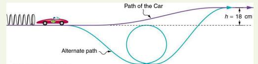
Figure 7.12 A toy car is pushed by a compressed spring and coasts up a slope. Assuming negligible friction, the potential energy in the spring is first completely converted to kinetic energy, and then to a combination of kinetic and gravitational potential energy as the car rises. The details of the path are unimportant because all forces are conservative—the car would have the same final speed if it took the alternate path shown.
