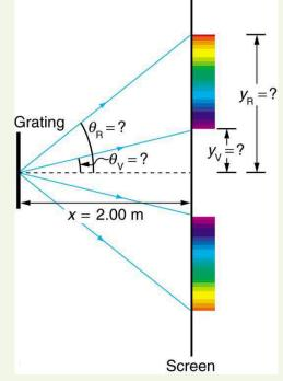
Figure 27.20 The diffraction grating considered in this example produces a rainbow of colors on a screen a distance x = 2.00 m from the grating. The distances along the screen are measured perpendicular to the *x* -direction. In other words, the rainbow pattern extends out of the page.
