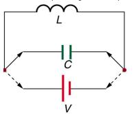
Figure 23.42 Through rapid switching of an inductor, 1.5 V batteries can be used to induce emfs of several thousand volts. This voltage can be used to store charge in a capacitor for later use, such as in a camera flash attachment.
