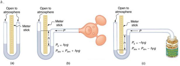
Figure 11.15 An open-tube manometer has one side open to the atmosphere. (a) Fluid depth must be the same on both sides, or the pressure each side exerts at the bottom will be unequal and there will be flow from the deeper side. (b) A positive gauge pressure  $P_g = h\rho g$  transmitted to one
