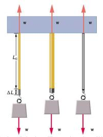
Figure 5.12 The same force, in this case a weight (*W*), applied to three different guitar strings of identical length produces the three different deformations shown as shaded segments. The string on the left is thin nylon, the one in the middle is thicker nylon, and the one on the right is steel.
