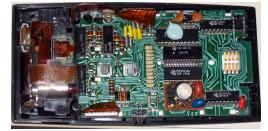
Figure 19.23 Energy stored in the large capacitor is used to preserve the memory of an electronic calculator when its batteries are charged. (credit: Kucharek, Wikimedia Commons)
