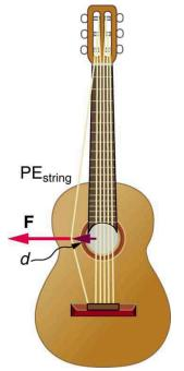
Figure 7.11 Work is done to deform the guitar string, giving it potential energy. When released, the potential energy is converted to kinetic energy and back to potential as the string oscillates back and forth. A very small fraction is dissipated as sound energy, slowly removing energy from the string.
