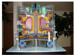
Figure 32.20 (a) Artist's rendition of ITER, a tokamak-type fusion reactor being built in southern France. It is hoped that this gigantic machine will reach the break-even point. Completion is scheduled for 2018. (credit: Stephan Mosel, Flickr)
