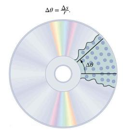
Figure 6.2 All points on a CD travel in circular arcs. The pits along a line from the center to the edge all move through the same angle  $\Delta \theta$  in a time  $\Delta t$ .
