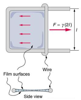
**Figure 11.28** Sliding wire device used for measuring surface tension; the device exerts a force to reduce the film's surface area. The force needed to hold the wire in place is  $F = \gamma L = \gamma(2l)$ , since there are *two* liquid surfaces attached to the wire. This force remains nearly constant as the film is stretched, until the film approaches its breaking point.
