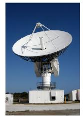
Figure 24.2 The electromagnetic waves sent and received by this 50-foot radar dish antenna at Kennedy Space Center in Florida are not visible, but help track expendable launch vehicles with high-definition imagery. The first use of this C-band radar dish was for the launch of the Atlas V rocket sending the New Horizons probe toward Pluto. (credit: NASA)
