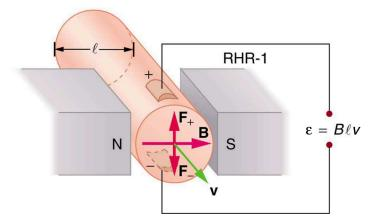
Figure 22.29 The Hall effect can be used to measure fluid flow in any fluid having free charges, such as blood. The Hall emf  $\varepsilon$  is measured across the tube perpendicular to the applied magnetic field and is proportional to the average velocity v.
