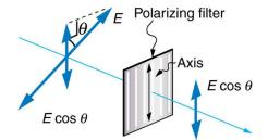
Figure 27.42 A polarizing filter transmits only the component of the wave parallel to its axis,  $E \cos \theta$ , reducing the intensity of any light not polarized parallel to its axis.
