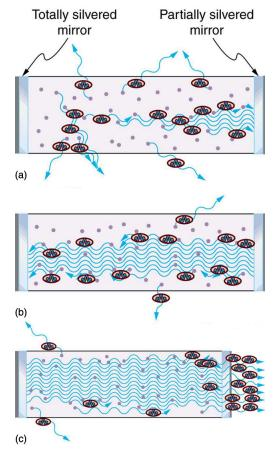
Figure 30.38 Typical laser construction has a method of pumping energy into the lasing material to produce a population inversion. (a) Spontaneous emission begins with some photons escaping and others stimulating further emissions. (b) and (c) Mirrors are used to enhance the probability of stimulated emission by passing photons through the material several times.
