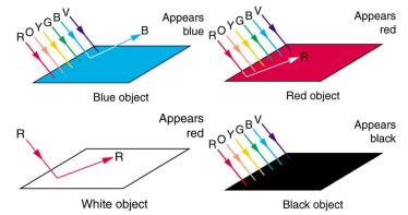
Figure 26.11 Absorption characteristics determine the true color of an object. Here, three objects are illuminated by white light, and one by pure red light. White is the equal mixture of all visible wavelengths; black is the absence of light.
