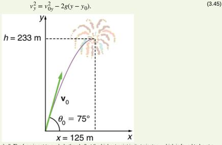
Figure 3.38 The trajectory of a fireworks shell. The fuse is set to explode the shell at the highest point in its trajectory, which is found to be at a height of 233 m and 125 m away horizontally.
