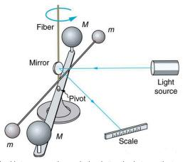
Figure 6.28 Cavendish used an apparatus like this to measure the gravitational attraction between the two suspended spheres (m) and the two on the stand (M) by observing the amount of torsion (twisting) created in the fiber. Distance between the masses can be varied to check the dependence of the force on distance. Modern experiments of this type continue to explore gravity.
