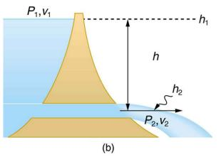
Figure 12.8 (a) Water gushes from the base of the Studen Kladenetz dam in Bulgaria. (credit: Kiril Kapustin; http://www.ImagesFromBulgaria.com) (b) In the absence of significant resistance, water flows from the reservoir with the same speed it would have if it fell the distance h without friction. This is an example of Torricelli's theorem.
