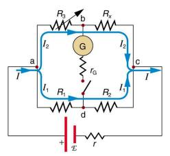
Figure 21.37 The Wheatstone bridge is used to calculate unknown resistances. The variable resistance  $R_3$  is adjusted until the galvanometer reads zero with the switch closed. This simplifies the circuit, allowing  $R_x$  to be calculated based on the *IR* drops as discussed in the text.
