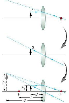
Figure 25.37 Ray tracing predicts the image location and size for an object held closer to a converging lens than its focal length. Ray 1 enters parallel to the axis and exits through the focal point on the opposite side, while ray 2 passes through the center of the lens without changing path. The two rays continue to diverge on the other side of the lens, but both appear to come from a common point, locating the upright, magnified, virtual image. This is a case 2 image.
