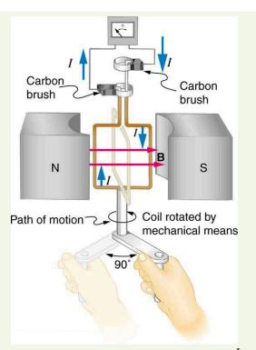
Figure 23.20 When this generator coil is rotated through one-fourth of a revolution, the magnetic flux  $\Phi$  changes from its maximum to zero, inducing an emf.
