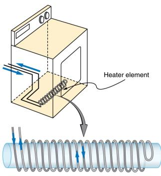
Figure 23.40 The heating coils of an electric clothes dryer can be counter-wound so that their magnetic fields cancel one another, greatly reducing the mutual inductance with the case of the dryer.
