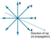
Figure 27.39 The slender arrow represents a ray of unpolarized light. The bold arrows represent the direction of polarization of the individual waves composing the ray. Since the light is unpolarized, the arrows point in all directions.
