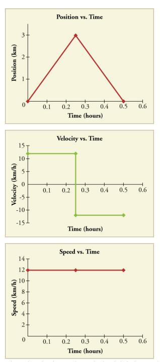
Figure 2.11 Position vs. time, velocity vs. time, and speed vs. time on a trip. Note that the velocity for the return trip is negative.
