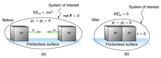
Figure 8.8 An inelastic one-dimensional two-object collision. Momentum is conserved, but internal kinetic energy is not conserved. (a) Two objects of equal mass initially head directly toward one another at the same speed. (b) The objects stick together (a perfectly inelastic collision), and so their final velocity is zero. The internal kinetic energy of the system changes in any inelastic collision and is reduced to zero in this example.
