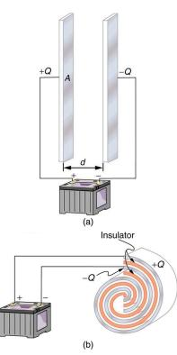
Figure 19.13 Both capacitors shown here were initially uncharged before being connected to a battery. They now have separated charges of +Q and -Q on their two halves. (a) A parallel plate capacitor. (b) A rolled capacitor with an insulating material between its two conducting sheets.
