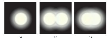
Figure 27.25 (a) Monochromatic light passed through a small circular aperture produces this diffraction pattern. (b) Two point light sources that are close to one another produce overlapping images because of diffraction. (c) If they are closer together, they cannot be resolved or distinguished.
