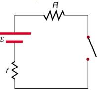
Figure 21.43 A switch is ordinarily in series with a resistance and voltage source. Ideally, the switch has nearly zero resistance when closed but has an extremely large resistance when open. (Note that in this diagram, the script E represents the voltage (or electromotive force) of the battery.)
