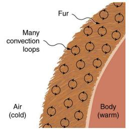
Figure 14.19 Fur is filled with air, breaking it up into many small pockets. Convection is very slow here, because the loops are so small. The low conductivity of air makes fur a very good lightweight insulator.
