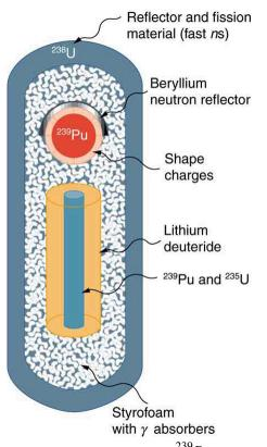
Figure 32.31 This schematic of a fusion bomb (H-bomb) gives some idea of how the  $^{239}$ Pu fission trigger is used to ignite fusion fuel. Neutrons and
