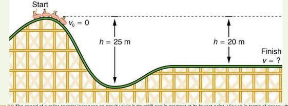
Figure 7.8 The speed of a roller coaster increases as gravity pulls it downhill and is greatest at its lowest point. Viewed in terms of energy, the roller-coaster-Earth system's gravitational potential energy is converted to kinetic energy. If work done by friction is negligible, all  $\Delta PE_g$  is
