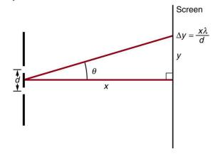
**Figure 27.56** The distance between adjacent fringes is  $\Delta y = x\lambda/d$ ,
