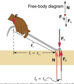
Figure 9.22 A nail puller is a lever with a large mechanical advantage. The external forces on the nail puller are represented by solid arrows. The force that the nail puller applies to the nail ( $\mathbf{F}_{o}$ ) is not a force on the nail puller. The reaction force the nail exerts back on the puller ( $\mathbf{F}_{n}$ ) is an external force and is equal and opposite to  $\mathbf{F}_{o}$ . The perpendicular lever arms of the input and output forces are  $l_{i}$  and  $l_{o}$ .
