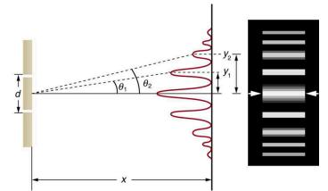
Figure 27.15 The interference pattern for a double slit has an intensity that falls off with angle. The photograph shows multiple bright and dark lines, or fringes, formed by light passing through a double slit.
