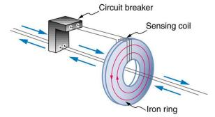
Figure 23.37 A GFI compares currents by using both to induce an emf in the same coil. If the currents are equal, they will induce equal but opposite emfs.
