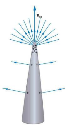
Figure 18.36 A very pointed conductor has a large charge concentration at the point. The electric field is very strong at the point and can exert a force large enough to transfer charge on or off the conductor. Lightning rods are used to prevent the buildup of large excess charges on structures and, thus, are pointed.
