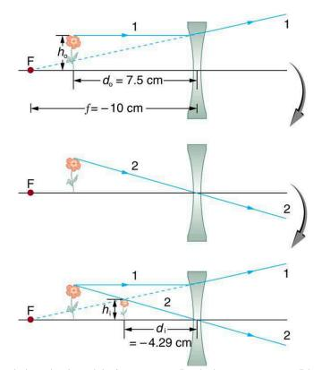
Figure 25.39 Ray tracing predicts the image location and size for a concave or diverging lens. Ray 1 enters parallel to the axis and is bent so that it appears to originate from the focal point. Ray 2 passes through the center of the lens without changing path. The two rays appear to come from a common point, locating the upright image. This is a case 3 image, which is closer to the lens than the object and smaller in height.
