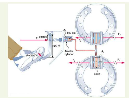
Figure 11.13 Hydraulic brakes use Pascal's principle. The driver exerts a force of 100 N on the brake pedal. This force is increased by the simple lever and again by the hydraulic system. Each of the identical slave cylinders receives the same pressure and, therefore, creates the same force output  $F_2$ . The circular cross-sectional areas of the master and slave cylinders are represented by  $A_1$  and  $A_2$ , respectively
