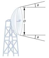
Figure 27.29 The beam produced by this microwave transmission antenna will spread out at a minimum angle  $\theta = 1.22 \lambda/D$  due to diffraction. It is impossible to produce a near-parallel beam, because the beam has a limited diameter.
