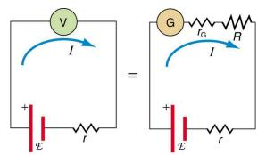
Figure 21.34 An analog voltmeter attached to a battery draws a small but nonzero current and measures a terminal voltage that differs from the emf of the battery. (Note that the script capital E symbolizes electromotive force, or emf.) Since the internal resistance of the battery is not known precisely, it is not possible to calculate the emf precisely.
