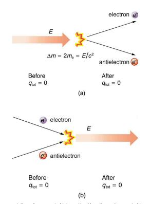
Figure 18.9 (a) When enough energy is present, it can be converted into matter. Here the matter created is an electron–antielectron pair. ( $m_e$  is the electron's mass.) The total charge before and after this event is zero. (b) When matter and antimatter collide, they annihilate each other; the total charge is conserved at zero before and after the annihilation.
