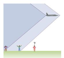
Figure 17.17 Two sonic booms, created by the nose and tail of an aircraft, are observed on the ground after the plane has passed by.
