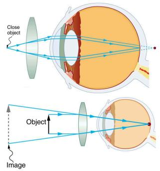
Figure 26.7 Correction of farsightedness uses a converging lens that compensates for the under convergence by the eye. The converging lens produces an image farther from the eye than the object, so that the farsighted person can see it clearly.
