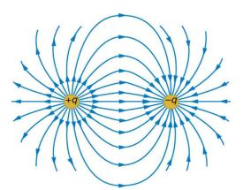
Figure 4.25 The electric force field between a positively charged particle and a negatively charged particle. When a positive test charge is placed in the field, the charge will experience a force in the direction of the force field lines.
