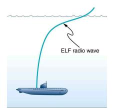
Figure 24.11 Very long wavelength radio waves are needed to reach this submarine, requiring extremely low frequency signals (ELF). Shorter wavelengths do not penetrate to any significant depth.
