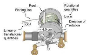
Figure 10.8 Fishing line coming off a rotating reel moves linearly. Example 10.3 and Example 10.4 consider relationships between rotational and linear quantities associated with a fishing reel.
