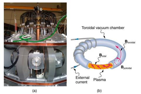
Figure 22.26 Tokamaks such as the one shown in the figure are being studied with the goal of economical production of energy by nuclear fusion. Magnetic fields in the doughnut-shaped device contain and direct the reactive charged particles. (credit: David Mellis, Flickr)
