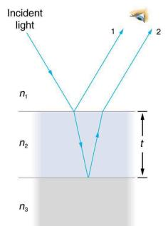
Figure 27.33 Light striking a thin film is partially reflected (ray 1) and partially refracted at the top surface. The refracted ray is partially reflected at the bottom surface and emerges as ray 2. These rays will interfere in a way that depends on the thickness of the film and the indices of refraction of the various media.
