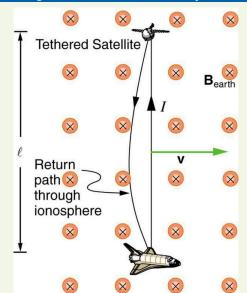
Figure 23.12 Motional emf as electrical power conversion for the space shuttle is the motivation for the Tethered Satellite experiment. A 5 kV emf was predicted to be induced in the 20 km long tether while moving at orbital speed in the Earth's magnetic field. The circuit is completed by a return path through the stationary ionosphere.
