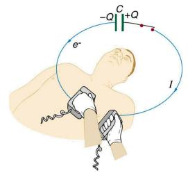
Figure 20.38 The capacitor in a defibrillation unit drives a current through the heart of a patient.
