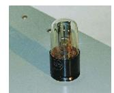
Figure 29.7 The photoelectric effect can be observed by allowing light to fall on the metal plate in this evacuated tube. Electrons ejected by the light are collected on the collector wire and measured as a current. A retarding voltage between the collector wire and plate can then be adjusted so as to determine the energy of the ejected electrons. For example, if it is sufficiently negative, no electrons will reach the wire. (credit: P.P. Urone)
