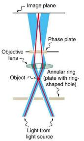
Figure 27.53 Simplified construction of a phase-contrast microscope. Phase differences between light passing through the object and background are produced by passing the rays through different parts of a phase plate. The light rays are superimposed in the image plane, producing contrast due to their interference.
