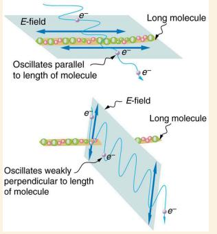
Figure 27.45 Artist's conception of an electron in a long molecule oscillating parallel to the molecule. The oscillation of the electron absorbs energy and reduces the intensity of the component of the EM wave that is parallel to the molecule.
