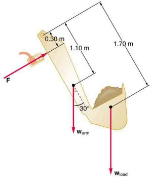
Figure 11.44 Hydraulic and mechanical lever systems are used in heavy machinery such as this back hoe.
