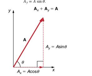
Figure 3.27 The magnitudes of the vector components  $A_x$  and  $A_y$  can be related to the resultant vector A and the angle  $\theta$  with trigonometric identities. Here we see that  $A_x = A \cos \theta$  and  $A_y = A \sin \theta$ .
