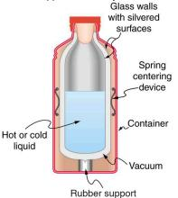
Figure 14.30 The construction of a thermos bottle is designed to inhibit all methods of heat transfer.
