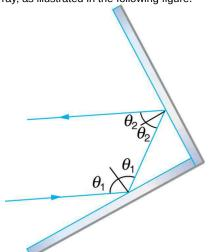
Figure 25.51 A corner reflector sends the reflected ray back in a direction parallel to the incident ray, independent of incoming direction.
