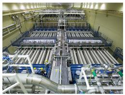
Figure 32.21 National Ignition Facility (CA). This image shows a laser bay where 192 laser beams will focus onto a small D-T target, producing fusion. (credit: Lawrence Livermore National Laboratory, Lawrence Livermore National Security, LLC, and the Department of Energy)
