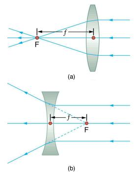
Figure 25.31 Thin lenses have the same focal length on either side. (a) Parallel light rays entering a converging lens from the right cross at its focal point on the left. (b) Parallel light rays entering a diverging lens from the right seem to come from the focal point on the right.
