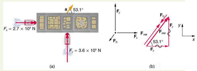
Figure 4.22 (a) A view from above of two tugboats pushing on a barge. (b) The free-body diagram for the ship contains only forces acting in the plane of the water. It omits the two vertical forces—the weight of the barge and the buoyant force of the water supporting it cancel and are not shown. Since the applied forces are perpendicular, the *x*- and *y*-axes are in the same direction as  $\mathbf{F}_x$  and  $\mathbf{F}_y$ . The problem quickly becomes a
