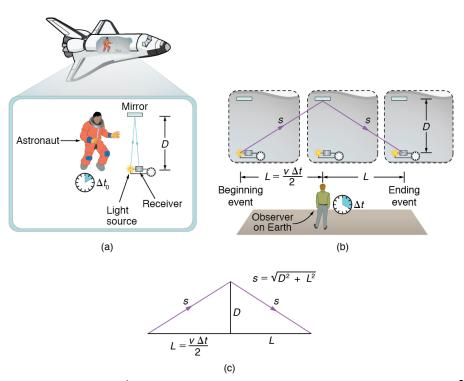
Figure 28.6 (a) An astronaut measures the time  $\Delta t_0$  for light to cross her ship using an electronic timer. Light travels a distance 2D in the astronaut's frame. (b) A person on the Earth sees the light follow the longer path 2s and take a longer time  $\Delta t$ . (c) These triangles are used to find the relationship between the two distances 2D and 2s.
