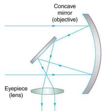
Figure 26.25 A two-element telescope composed of a mirror as the objective and a lens for the eyepiece is shown. This telescope forms an image in the same manner as the two-convex-lens telescope already discussed, but it does not suffer from chromatic aberrations. Such telescopes can gather more light, since larger mirrors than lenses can be constructed.
