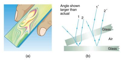
Figure 27.34 (a) The rainbow color bands are produced by thin film interference in the air between the two glass slides. (b) Schematic of the paths taken by rays in the wedge of air between the slides.
