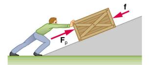
Figure 7.16 A person pushes a crate up a ramp, doing work on the crate. Friction and gravitational force (not shown) also do work on the crate; both forces oppose the person's push. As the crate is pushed up the ramp, it gains mechanical energy, implying that the work done by the person is greater than the work done by friction.
