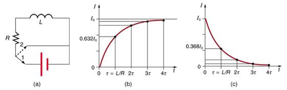
Figure 23.44 (a) An *RL* circuit with a switch to turn current on and off. When in position 1, the battery, resistor, and inductor are in series and a current is established. In position 2, the battery is removed and the current eventually stops because of energy loss in the resistor. (b) A graph of current growth versus time when the switch is moved to position 1. (c) A graph of current decay when the switch is moved to position 2.
