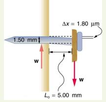
Figure 5.17 Side view of a nail with a picture hung from it. The nail flexes very slightly (shown much larger than actual) because of the shearing effect of the supported weight. Also shown is the upward force of the wall on the nail, illustrating that there are equal and opposite forces applied across opposite cross sections of the nail. See Example 5.5 for a calculation of the mass of the picture.
