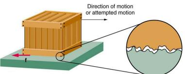
Figure 5.2 Frictional forces, such as f, always oppose motion or attempted motion between surfaces in contact. Friction arises in part because of the
