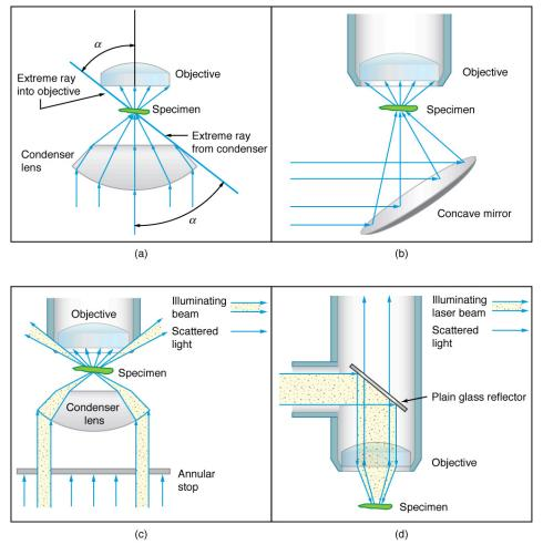
Figure 26.20 Illumination of a specimen in a microscope. (a) Transmitted light from a condenser lens. (b) Transmitted light from a mirror condenser. (c) Dark field illumination by scattering (the illuminating beam misses the objective lens). (d) High magnification illumination with reflected light – normally laser light.
