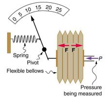
Figure 11.14 This aneroid gauge utilizes flexible bellows connected to a mechanical indicator to measure pressure.
