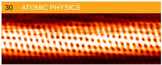
Figure 30.1 Individual carbon atoms are visible in this image of a carbon nanotube made by a scanning tunneling electron microscope. (credit: Taner Yildirim, National Institute of Standards and Technology, via Wikimedia Commons)
