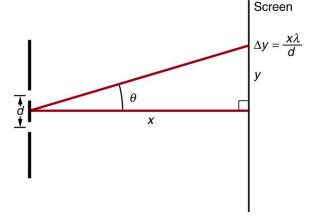
**Figure 27.57** The distance between adjacent fringes is  $\Delta y = x\lambda/d$ ,
