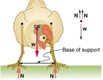
Figure 9.17 The center of gravity of a chicken is below the hip joints. The chicken is in stable equilibrium. The body of the chicken is supported from above by the hips and acts as a pendulum between them.
