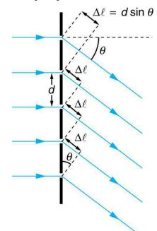
Figure 27.19 Diffraction grating showing light rays from each slit traveling in the same direction. Each ray travels a different distance to reach a common point on a screen (not shown). Each ray travels a distance  $d \sin \theta$  different from that of its neighbor.
