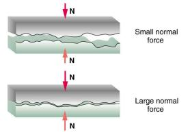
Figure 5.5 Two rough surfaces in contact have a much smaller area of actual contact than their total area. When there is a greater normal force as a result of a greater applied force, the area of actual contact increases as does friction.
