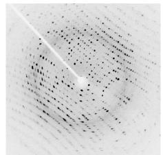
Figure 30.29 X-ray diffraction from the crystal of a protein, hen egg lysozyme, produced this interference pattern. Analysis of the pattern yields information about the structure of the protein. (credit: Del45, Wikimedia Commons)
