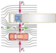
Figure 12.4 An overhead view of a car passing a truck on a highway. Air passing between the vehicles flows in a narrower channel and must increase its speed ( $v_2$  is greater than  $v_1$ ), causing the pressure between them to drop ( $P_i$  is less than  $P_0$ ). Greater pressure on the outside pushes the car and truck together.
