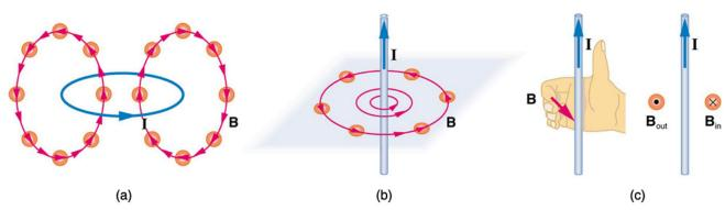
Figure 22.16 Small compasses could be used to map the fields shown here. (a) The magnetic field of a circular current loop is similar to that of a bar magnet. (b) A long and straight wire creates a field with magnetic field lines forming circular loops. (c) When the wire is in the plane of the paper, the field is perpendicular to the paper. Note that the symbols used for the field pointing inward (like the tail of an arrow) and the field pointing outward (like the tip of an arrow).
