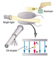
**Figure 30.9** The Millikan oil drop experiment produced the first accurate direct measurement of the charge on electrons, one of the most fundamental constants in nature. Fine drops of oil become charged when sprayed. Their movement is observed between metal plates with a potential applied to oppose the gravitational force. The balance of gravitational and electric forces allows the calculation of the charge on a drop. The charge is found to be
