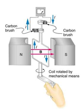
Figure 23.5 Rotation of a coil in a magnetic field produces an emf. This is the basic construction of a generator, where work done to turn the coil is converted to electric energy. Note the generator is very similar in construction to a motor.
