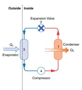
Figure 15.28 A simple heat pump has four basic components: (1) condenser, (2) expansion valve, (3) evaporator, and (4) compressor. In the heating mode, heat transfer  $Q_c$  occurs to the working fluid in the evaporator (3) from the colder outdoor air, turning it into a gas. The electrically driven
