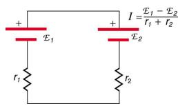
Figure 21.17 These two voltage sources are connected in series with their emfs in opposition. Current flows in the direction of the greater emf and is limited to  $I = \frac{(\text{emf}_1 - \text{emf}_2)}{r_1 + r_2}$  by the sum of the internal resistances. (Note that each emf is represented by script E in the figure.) A battery
