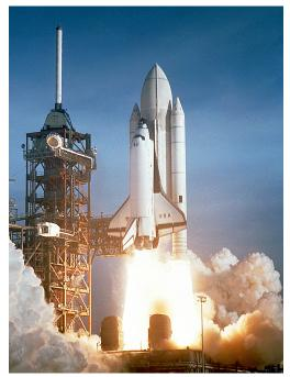
Figure 8.14 The space shuttle had a number of reusable parts. Solid fuel boosters on either side were recovered and refueled after each flight, and the entire orbiter returned to Earth for use in subsequent flights. The large liquid fuel tank was expended. The space shuttle was a complex assemblage of technologies, employing both solid and liquid fuel and pioneering ceramic tiles as reentry heat shields. As a result, it permitted multiple launches as opposed to single-use rockets. (credit: NASA)
