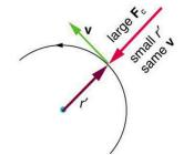
Figure 6.11 The frictional force supplies the centripetal force and is numerically equal to it. Centripetal force is perpendicular to velocity and causes uniform circular motion. The larger the  $F_c$ , the smaller the radius of curvature r and the sharper the curve. The second curve has the same v, but the second curve has the same r'.
