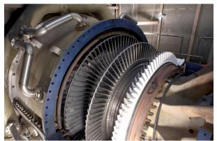
Figure 23.24 Steam turbine/generator. The steam produced by burning coal impacts the turbine blades, turning the shaft which is connected to the generator. (credit: Nabonaco, Wikimedia Commons)
