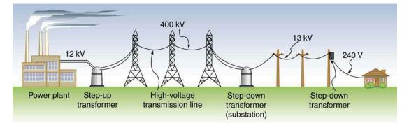
**Figure 23.27** Transformers change voltages at several points in a power distribution system. Electric power is usually generated at greater than 10 kV, and transmitted long distances at voltages over 200 kV—sometimes as great as 700 kV—to limit energy losses. Local power distribution to neighborhoods or industries goes through a substation and is sent short distances at voltages ranging from 5 to 13 kV. This is reduced to 120, 240, or 480 V for safety at the individual user site.
