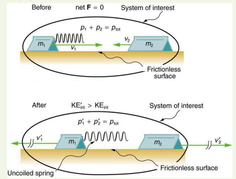
Figure 8.10 An air track is nearly frictionless, so that momentum is conserved. Motion is one-dimensional. In this collision, examined in Example 8.6, the potential energy of a compressed spring is released during the collision and is converted to internal kinetic energy.
