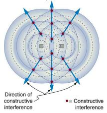
Figure 24.26 An overhead view of two radio broadcast antennas sending the same signal, and the interference pattern they produce.
