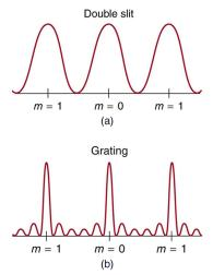
Figure 27.18 Idealized graphs of the intensity of light passing through a double slit (a) and a diffraction grating (b) for monochromatic light. Maxima can be produced at the same angles, but those for the diffraction grating are narrower and hence sharper. The maxima become narrower and the regions between darker as the number of slits is increased.
