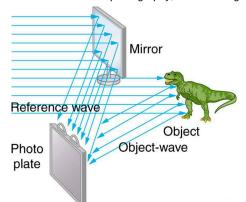
Figure 30.44 Production of a hologram. Single-wavelength coherent light from a laser produces a well-defined interference pattern on a piece of film. The laser beam is split by a partially silvered mirror, with part of the light illuminating the object and the remainder shining directly on the film.
