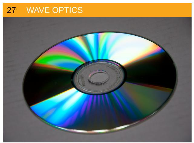
Figure 27.1 The colors reflected by this compact disc vary with angle and are not caused by pigments. Colors such as these are direct evidence of the wave character of light. (credit: Infopro, Wikimedia Commons)
