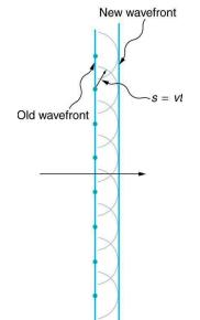
Figure 27.5 Huygens's principle applied to a straight wavefront. Each point on the wavefront emits a semicircular wavelet that moves a distance S = vt. The new wavefront is a line tangent to the wavelets.
