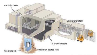
Figure 32.12 A food irradiation plant has a conveyor system to pass items through an intense radiation field behind thick shielding walls. The  $\gamma$
