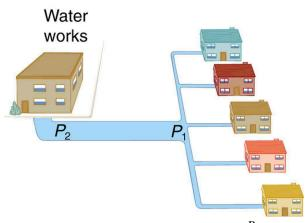
Figure 12.15 During times of heavy use, there is a significant pressure drop in a water main, and  $P_1$  supplied to users is significantly less than  $P_2$  created at the water works. If the flow is very small, then the pressure drop is negligible, and  $P_2 \approx P_1$ .
