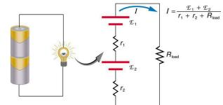
Figure 21.18 This schematic represents a flashlight with two cells (voltage sources) and a single bulb (load resistance) in series. The current that flows
