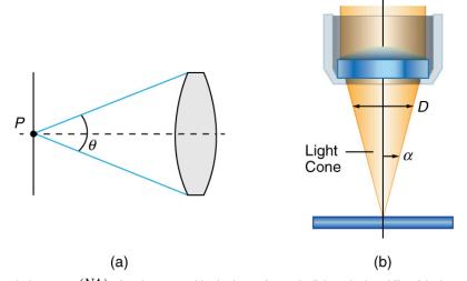
Figure 26.17 (a) The numerical aperture (NA) of a microscope objective lens refers to the light-gathering ability of the lens and is calculated using half the angle of acceptance  $\theta$ . (b) Here,  $\alpha$  is half the acceptance angle for light rays from a specimen entering a camera lens, and D is the diameter of the aperture that controls the light entering the lens.
