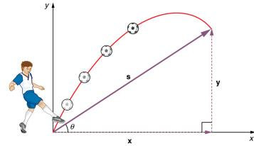
Figure 3.36 The total displacement **s** of a soccer ball at a point along its path. The vector **s** has components **x** and **y** along the horizontal and vertical axes. Its magnitude is s, and it makes an angle  $\theta$  with the horizontal.
