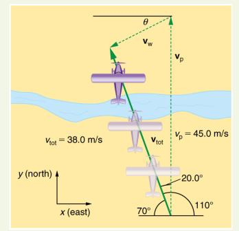
Figure 3.47 An airplane is known to be heading north at 45.0 m/s, though its velocity relative to the ground is 38.0 m/s at an angle west of north. What is the speed and direction of the wind?
