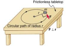
Figure 10.11 An object is supported by a horizontal frictionless table and is attached to a pivot point by a cord that supplies centripetal force. A force F is applied to the object perpendicular to the radius r, causing it to accelerate about the pivot point. The force is kept perpendicular to r.
