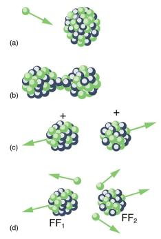
Figure 32.23 Neutron-induced fission is shown. First, energy is put into this large nucleus when it absorbs a neutron. Acting like a struck liquid drop, the nucleus deforms and begins to narrow in the middle. Since fewer nucleons are in contact, the repulsive Coulomb force is able to break the nucleus into two parts with some neutrons also flying away.
