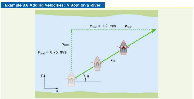
Figure 3.46 A boat attempts to travel straight across a river at a speed 0.75 m/s. The current in the river, however, flows at a speed of 1.20 m/s to the right.
