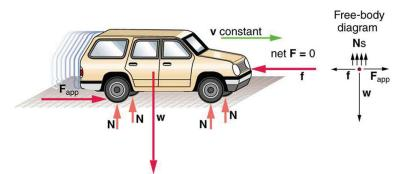
Figure 9.3 This car is in dynamic equilibrium because it is moving at constant velocity. There are horizontal and vertical forces, but the net external force in any direction is zero. The applied force  $F_{app}$  between the tires and the road is balanced by air friction, and the weight of the car is supported by the normal forces, here shown to be equal for all four tires.
