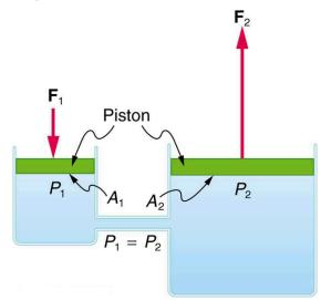
Figure 11.12 A typical hydraulic system with two fluid-filled cylinders, capped with pistons and connected by a tube called a hydraulic line. A downward force  $F_1$  on the left piston creates a pressure that is transmitted undiminished to all parts of the enclosed fluid. This results in an upward force  $F_2$  on the right piston that is larger than  $F_1$  because the right piston has a larger area.
