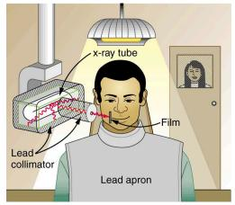
Figure 32.9 A lead apron is placed over the dental patient and shielding surrounds the x-ray tube to limit exposure to tissue other than the tissue that is being imaged. Fast films limit the time needed to obtain images, reducing exposure to the imaged tissue. The technician stands a few meters away behind a lead-lined door with a lead glass window, reducing her occupational exposure.
