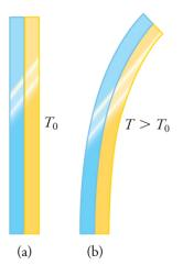
Figure 13.3 The curvature of a bimetallic strip depends on temperature. (a) The strip is straight at the starting temperature, where its two components have the same length. (b) At a higher temperature, this strip bends to the right, because the metal on the left has expanded more than the metal on the right.
