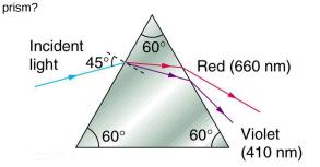
Figure 25.57 This prism will disperse the white light into a rainbow of colors. The incident angle is  $45.0^{\circ}$ , and the angles at which the red and violet light emerge are  $\theta_{\rm R}$  and  $\theta_{\rm V}$ .
