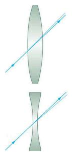
Figure 25.32 The light ray through the center of a thin lens is deflected by a negligible amount and is assumed to emerge parallel to its original path (shown as a shaded line).
