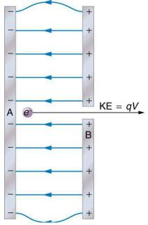
Figure 19.4 A typical electron gun accelerates electrons using a potential difference between two metal plates. The energy of the electron in electron volts is numerically the same as the voltage between the plates. For example, a 5000 V potential difference produces 5000 eV electrons.
