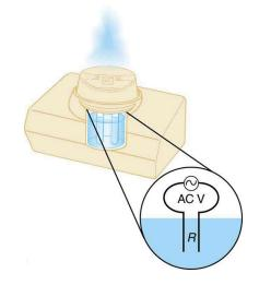
Figure 20.42 This cold vaporizer passes current directly through water, vaporizing it directly with relatively little temperature increase.
