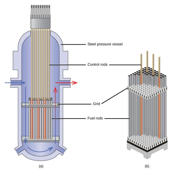
**Figure 21.20** The nuclear reactor core shown in (a) contains the fuel and control rod assembly shown in (b). (credit: modification of work by E. Generalic, http://glossary.periodni.com/glossary.php?en=control+rod)
