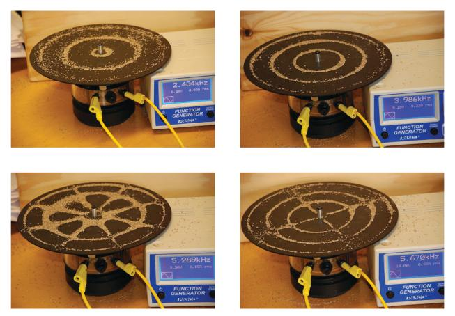
**Figure 6.8** Two-dimensional standing waves can be visualized on a vibrating surface. The surface has been sprinkled with a powder that collects near the nodal lines. There are two types of nodes visible: radial nodes (circles) and angular nodes (radii).
