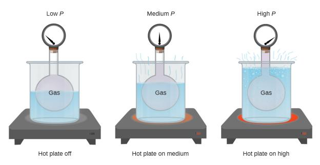
**Figure 9.10** The effect of temperature on gas pressure: When the hot plate is off, the pressure of the gas in the sphere is relatively low. As the gas is heated, the pressure of the gas in the sphere increases.
