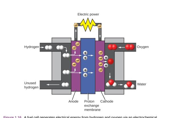
**Figure 1.16** A fuel cell generates electrical energy from hydrogen and oxygen via an electrochemical process and produces only water as the waste product.
