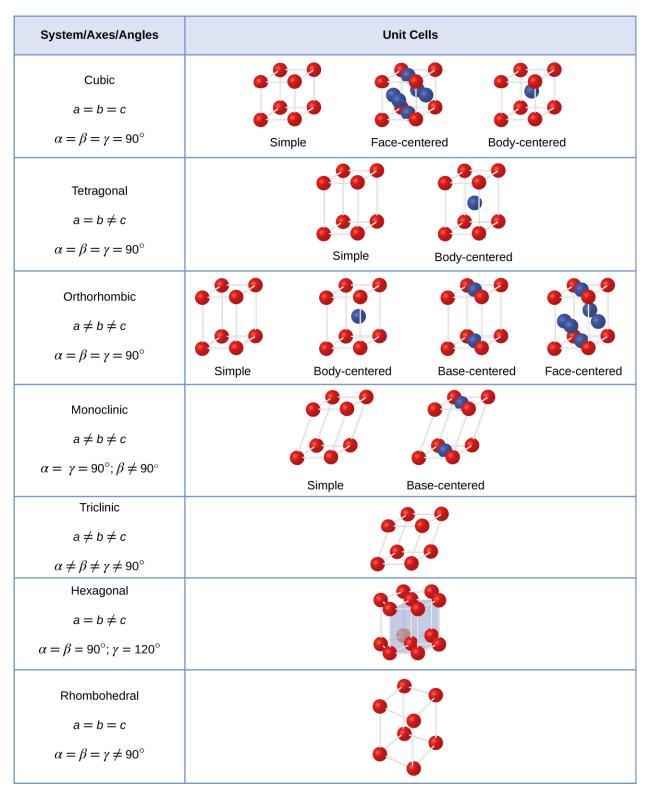
Figure 10.56 There are seven different lattice systems and 14 different unit cells.
