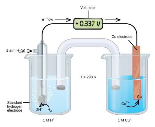
**Figure 17.6** A cell permitting experimental measurement of the standard electrode potential for the half-reaction  $Cu^{2+}(aq) + 2e^{-} \longrightarrow Cu(s)$
