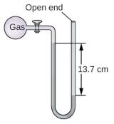
**16.** The pressure of a sample of gas is measured at sea level with an open-end mercury manometer. Assuming atmospheric pressure is 760 mm Hg, determine the pressure of the gas in:
