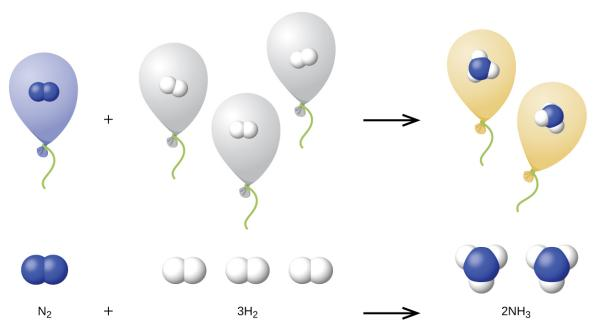
Figure 9.23 One volume of  $N_2$  combines with three volumes of  $H_2$  to form two volumes of  $NH_3$ .
