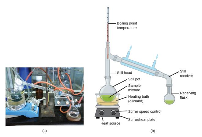
**Figure 11.19** A typical laboratory distillation unit is shown in (a) a photograph and (b) a schematic diagram of the components. (credit a: modification of work by "Rifleman82"/Wikimedia commons; credit b: modification of work by "Slashme"/Wikimedia Commons)
