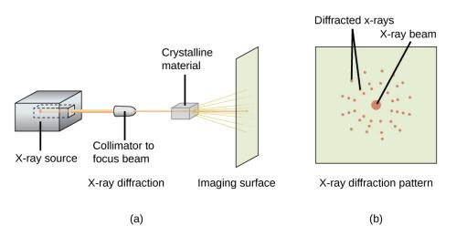
**Figure 10.65** (a) In a diffractometer, a beam of X-rays strikes a crystalline material, producing (b) an X-ray diffraction pattern that can be analyzed to determine the crystal structure.
