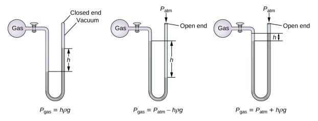
**Figure 9.5** A manometer can be used to measure the pressure of a gas. The (difference in) height between the liquid levels (*h*) is a measure of the pressure. Mercury is usually used because of its large density.
