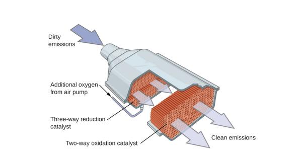
**Figure 12.24** A catalytic converter allows for the combustion of all carbon-containing compounds to carbon dioxide, while at the same time reducing the output of nitrogen oxide and other pollutants in emissions from gasoline-burning engines.
