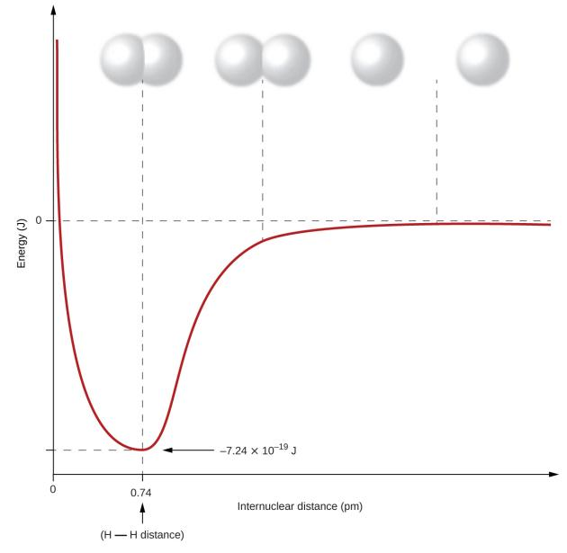
**Figure 7.4** The potential energy of two separate hydrogen atoms (right) decreases as they approach each other, and the single electrons on each atom are shared to form a covalent bond. The bond length is the internuclear distance at which the lowest potential energy is achieved.
