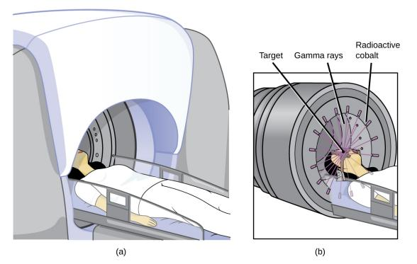
**Figure 21.26** The cartoon in (a) shows a cobalt-60 machine used in the treatment of cancer. The diagram in (b) shows how the gantry of the Co-60 machine swings through an arc, focusing radiation on the targeted region (tumor) and minimizing the amount of radiation that passes through nearby regions.
