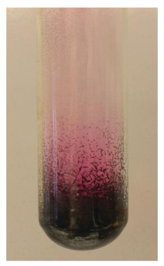
**Figure 10.27** Sublimation of solid iodine in the bottom of the tube produces a purple gas that subsequently deposits as solid iodine on the colder part of the tube above. (credit: modification of work by Mark Ott)
