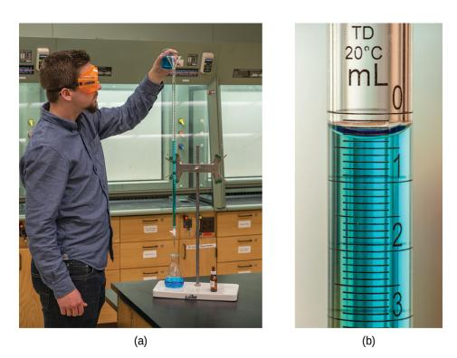
**Figure 4.16** (a) A student fills a buret in preparation for a titration analysis. (b) A typical buret permits volume measurements to the nearest 0.01 mL. (credit a: modification of work by Mark Blaser and Matt Evans; credit b: modification of work by Mark Blaser and Matt Evans)
