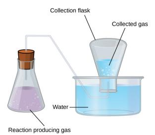
**Figure 9.21** When a reaction produces a gas that is collected above water, the trapped gas is a mixture of the gas produced by the reaction and water vapor. If the collection flask is appropriately positioned to equalize the water levels both within and outside the flask, the pressure of the trapped gas mixture will equal the atmospheric pressure outside the flask (see the earlier discussion of manometers).
