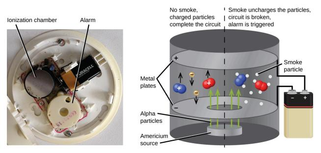
**Figure 21.29** Inside a smoke detector, Am-241 emits α particles that ionize the air, creating a small electric current. During a fire, smoke particles impede the flow of ions, reducing the current and triggering an alarm. (credit a: modification of work by "Muffet"/Wikimedia Commons)
