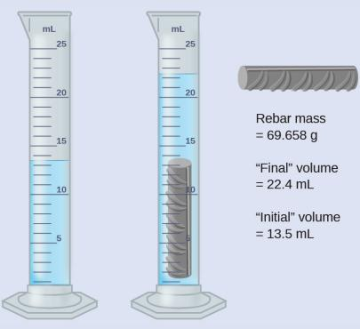
(a) Use these values to determine the density of this piece of rebar.
