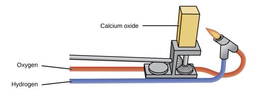
Figure 18.43 Calcium oxide has many industrial uses. When it is heated at high temperatures, it emits an intense white light.
