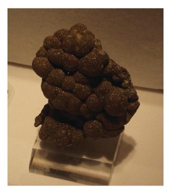
**Figure 19.8** Blister copper is obtained during the conversion of copper-containing ore into pure copper. (credit: "Tortie tude"/Wikimedia Commons)
