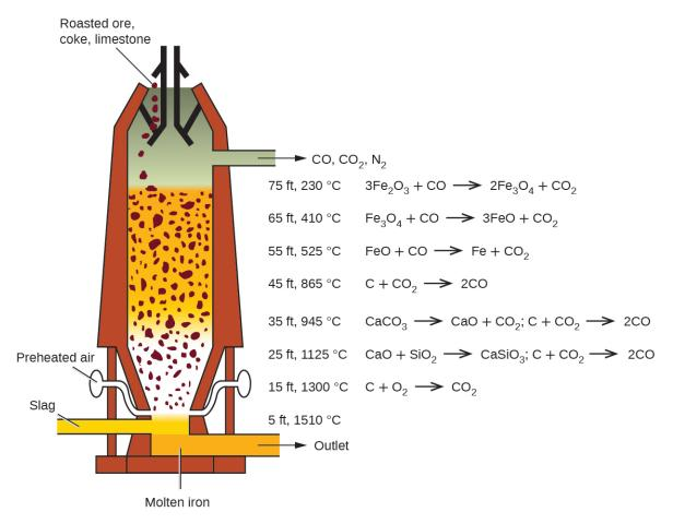
**Figure 19.6** Within a blast furnace, different reactions occur in different temperature zones. Carbon monoxide is generated in the hotter bottom regions and rises upward to reduce the iron oxides to pure iron through a series of reactions that take place in the upper regions.
