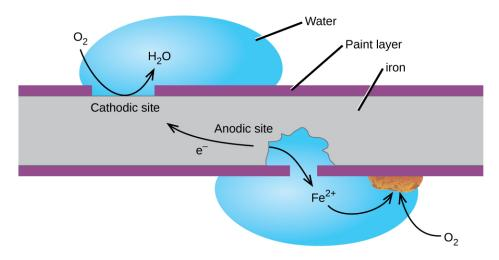
**Figure 17.16** Corrosion can occur when a painted iron or steel surface is exposed to the environment by a scratch through the paint. A galvanic cell results that may be approximated by the simplified cell schematic  $Fe(s) | Fe^{2+}(aq) | |O_2(aq), H_2O(l) | Fe(s).$
