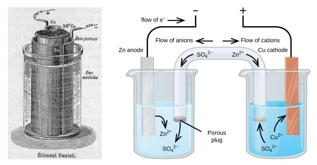
**Figure 17.8** Illustration of a Daniell cell taken from a 1904 journal publication (left) along with a simplified illustration depicting the electrochemistry of the cell (right). The 1904 design used a porous clay pot to both contain one of the half-cell's content and to serve as a salt bridge to the other half-cell.
