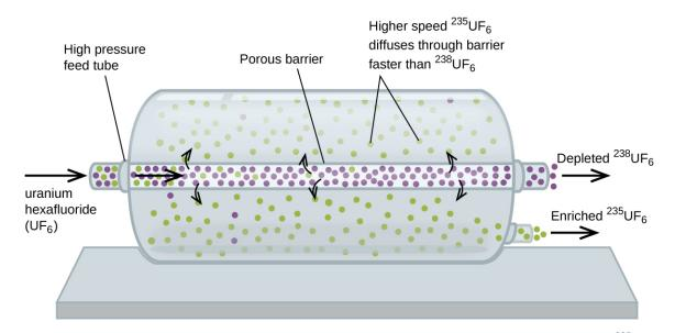
**Figure 9.30** In a diffuser, gaseous UF<sub>6</sub> is pumped through a porous barrier, which partially separates  ${}^{235}$ UF<sub>6</sub> from  ${}^{238}$ UF<sub>6</sub> The UF<sub>6</sub> must pass through many large diffuser units to achieve sufficient enrichment in  ${}^{235}$ U.
