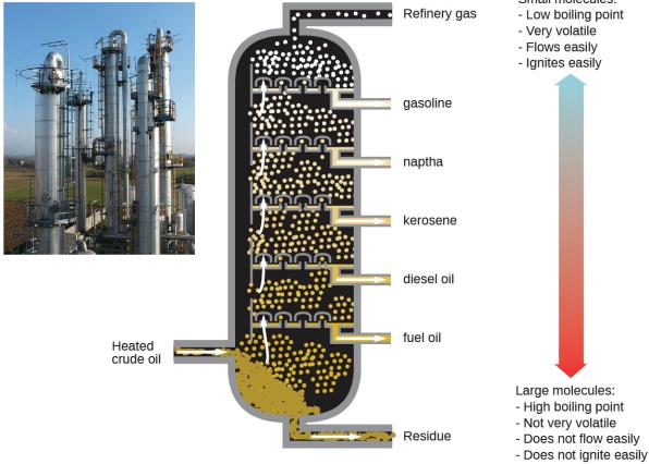
**Figure 11.20** Crude oil is a complex mixture that is separated by large-scale fractional distillation to isolate various simpler mixtures.
