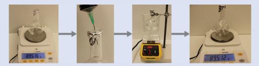
**Figure 9.19** When the volatile liquid in the flask is heated past its boiling point, it becomes gas and drives air out of the flask. At  $t_{l} \rightarrow g$ , the flask is filled with volatile liquid gas at the same pressure as the atmosphere. If the flask is then cooled to room temperature, the gas condenses and the mass of the gas that filled the flask, and is now liquid, can be measured. (credit: modification of work by Mark Ott)
