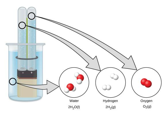
**Figure 18.26** The electrolysis of water produces hydrogen and oxygen. Because there are twice as many hydrogen atoms as oxygen atoms and both elements are diatomic, there is twice the volume of hydrogen produced at the cathode as there is oxygen produced at the anode.
