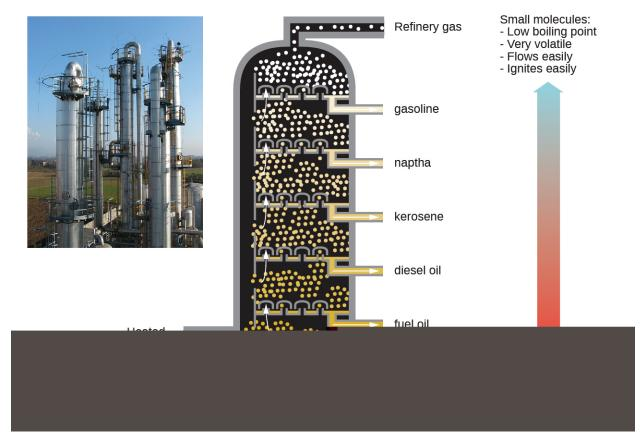
**Figure 20.6** In a column for the fractional distillation of crude oil, oil heated to about 425 °C in the furnace vaporizes when it enters the base of the tower. The vapors rise through bubble caps in a series of trays in the tower. As the vapors gradually cool, fractions of higher, then of lower, boiling points condense to liquids and are drawn off. (credit left: modification of work by Luigi Chiesa)
