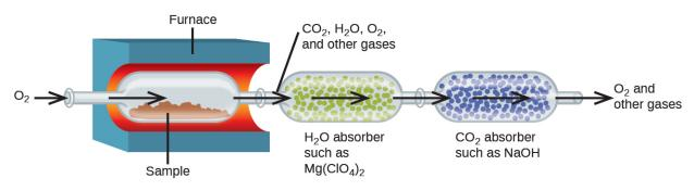
**Figure 4.18** This schematic diagram illustrates the basic components of a combustion analysis device for determining the carbon and hydrogen content of a sample.
