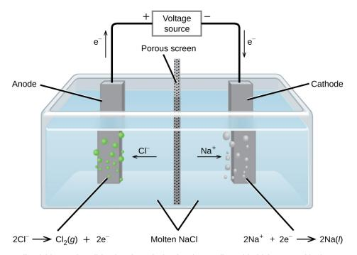
**Figure 17.18** Cells of this sort (a cell for the electrolysis of molten sodium chloride) are used in the *Downs process* for production of sodium and chlorine, and they typically use iron cathodes and carbon anodes.
