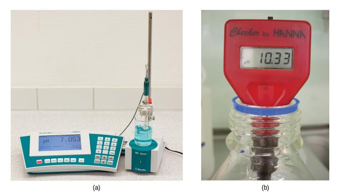
**Figure 14.4** (a) A research-grade pH meter used in a laboratory can have a resolution of 0.001 pH units, an accuracy of ± 0.002 pH units, and may cost in excess of \$1000. (b) A portable pH meter has lower resolution (0.01 pH units), lower accuracy (± 0.2 pH units), and a far lower price tag. (credit b: modification of work by Jacopo Werther)
