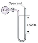
**15.** The pressure of a sample of gas is measured at sea level with an open-end mercury manometer. Assuming atmospheric pressure is 760.0 mm Hg, determine the pressure of the gas in:
