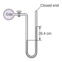
**14.** The pressure of a sample of gas is measured with an open-end manometer, partially shown to the right. The liquid in the manometer is mercury. Assuming atmospheric pressure is 29.92 in. Hg, determine the pressure of the gas in:
