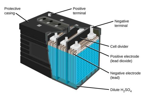
Figure 17.13 The lead acid battery in your automobile consists of six cells connected in series to give 12 V.
