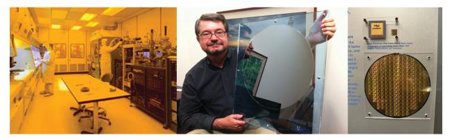
**Figure 18.1** Purity is extremely important when preparing silicon wafers. Technicians in a cleanroom prepare silicon without impurities (left). The CEO of VLSI Research, Don Hutcheson, shows off a pure silicon wafer (center). A silicon wafer covered in Pentium chips is an enlarged version of the silicon wafers found in many electronics used today (right). (credit middle: modification of work by "Intel Free Press"/Flickr; credit right: modification of work by Naotake Murayama)
