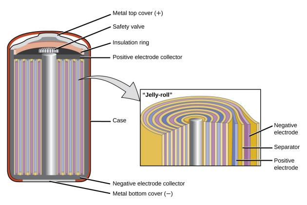
**Figure 17.11** NiCd batteries use a "jelly-roll" design that significantly increases the amount of current the battery can deliver as compared to a similar-sized alkaline battery.
