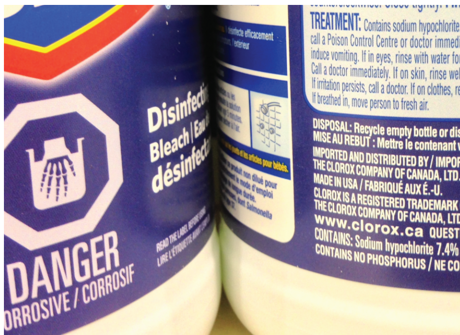
Figure 3.17 Liquid bleach is an aqueous solution of sodium hypochlorite (NaOCl). This brand has a concentration of 7.4% NaOCl by mass.
